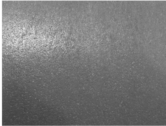
Figure 4. Wear surface of a HSS A roll operating in R4 and R5 stands
