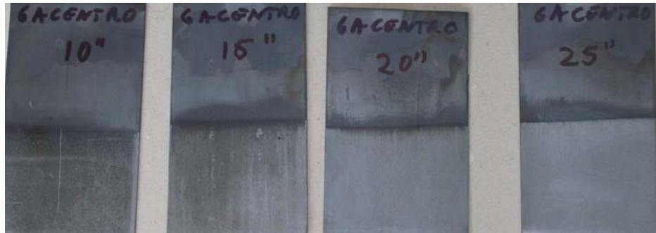
Figure 4. Example of pickled samples at different pickling time.
