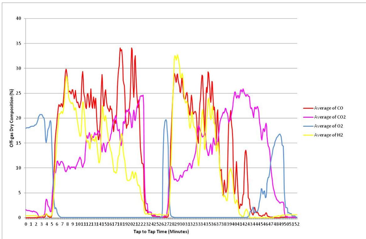
**Figure 3.** Typical off-gas chemistry of a two charge heat showing high concentration of CO and H<sub>2</sub> in melt phase.
