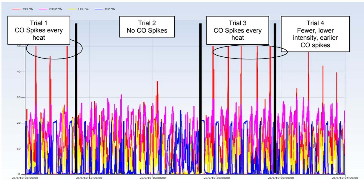
**Figure 9.** Series of heats during trials to improve bath mixing showing a cessation of CO spikes in trial 2 (removal of 1<sup>st</sup> charge carbon) and reduced CO spikes in trial 4 (1<sup>st</sup> charge super heat).
