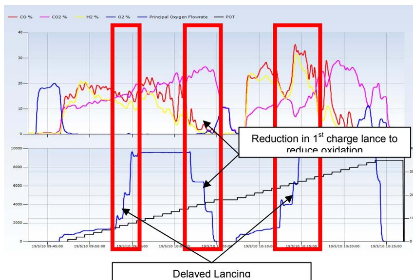
Figure 6. Modified lancing practice after off-gas analysis for ppmO<sub>2</sub> reduction.
