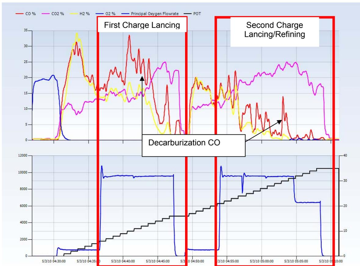
**Figure 4.** Off-gas and lancing timing showing significantly more evolution of carbon from the bath during first charge than during refining.
