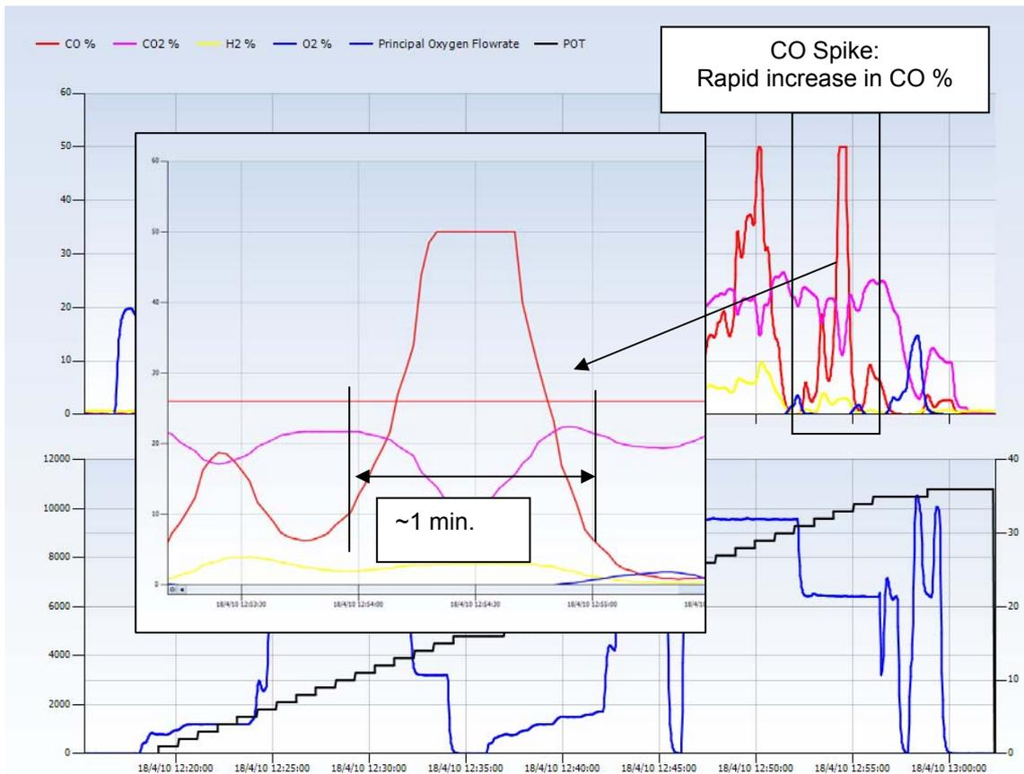
**Figure 7.** Close-up of CO spike showing long duration of CO generation indicating carbon boil.
