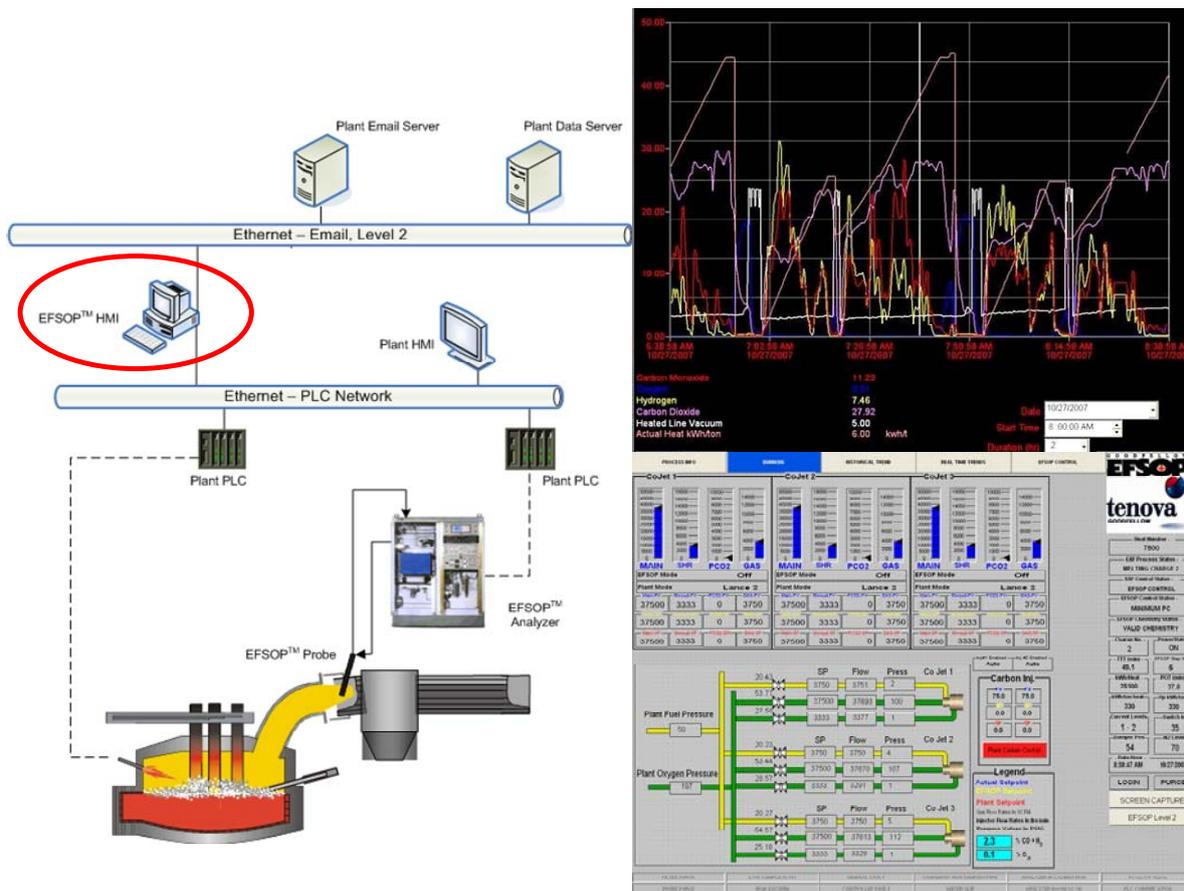
Figure 2. Schematic of EFSOP<sup>®</sup> System in plant Level 1 and Level 2 Ethernet network and screenshots of typical HMI.
