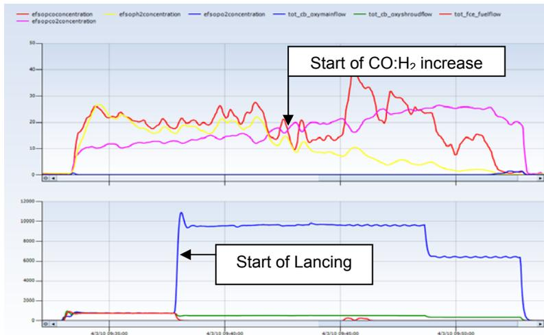
Figure 5. Solid scrap lancing at start of refining phase extends for 4 minutes.
