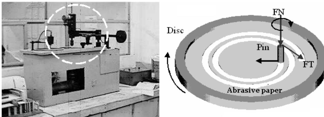
**Figure 2** – An illustration of pin-on-disk test.<sup>[11]</sup>
