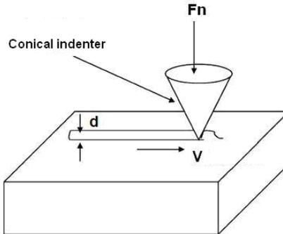
**Figure 4** – An illustration of a scratch test.  $F_n$  is the normal load,  $d$  is the size of the grove and  $V$  is the velocity of the translation motion.<sup>[20]</sup>
