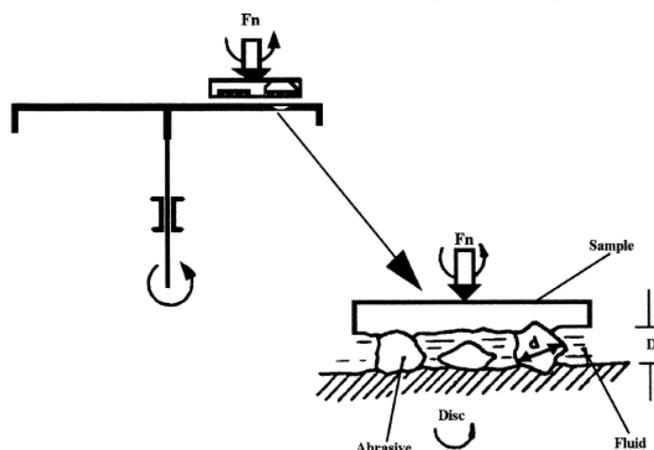
**Figure 1** – An illustration of LTM test.<sup>[6]</sup>  $F_n$  is the normal force.
