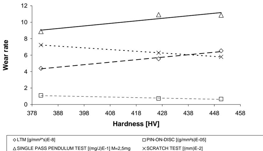
**Figure 5** – Wear rate behavior comparison among pin-on-disk, LTM, single pass pendulum and scratch test for white cast irons alloys.
