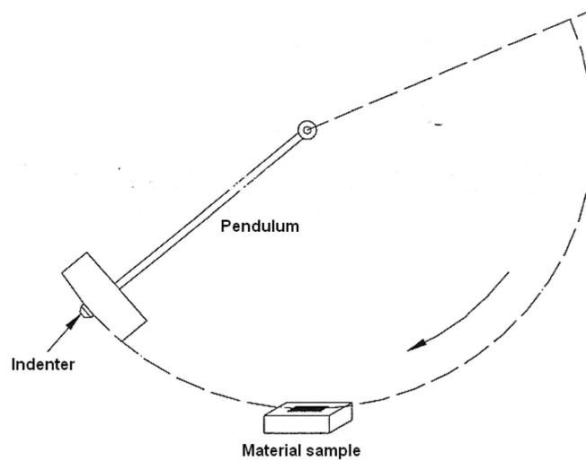
**Figure 3** – Illustration of a single pass pendulum test.<sup>[16]</sup>
