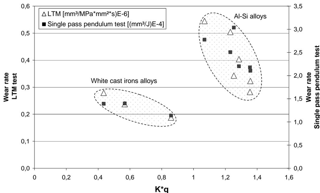
**Figure 10** – Wear rate behavior of single pass pendulum and LTM test as a function of the  $k \cdot q$  product.
