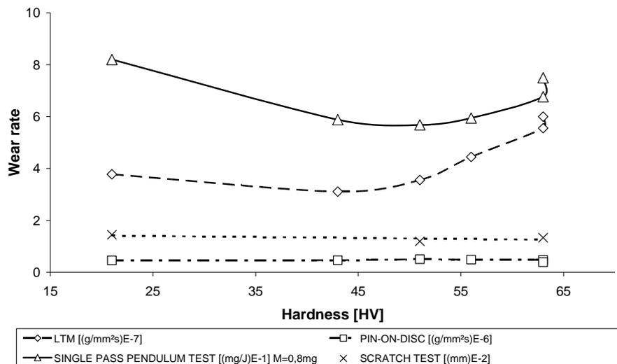
**Figure 6** - Wear rate behavior comparison among pin-on-disk, LTM, single pass pendulum and scratch test for Al-Si alloys.
