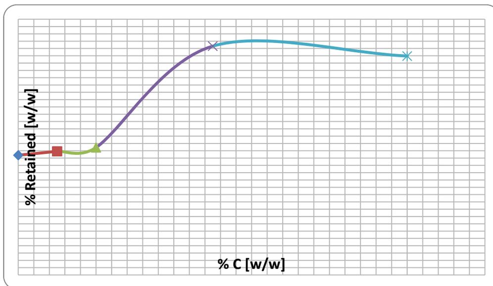
Figure 7. Mass percent retained of tumbler test depending on the graphite concentration.
