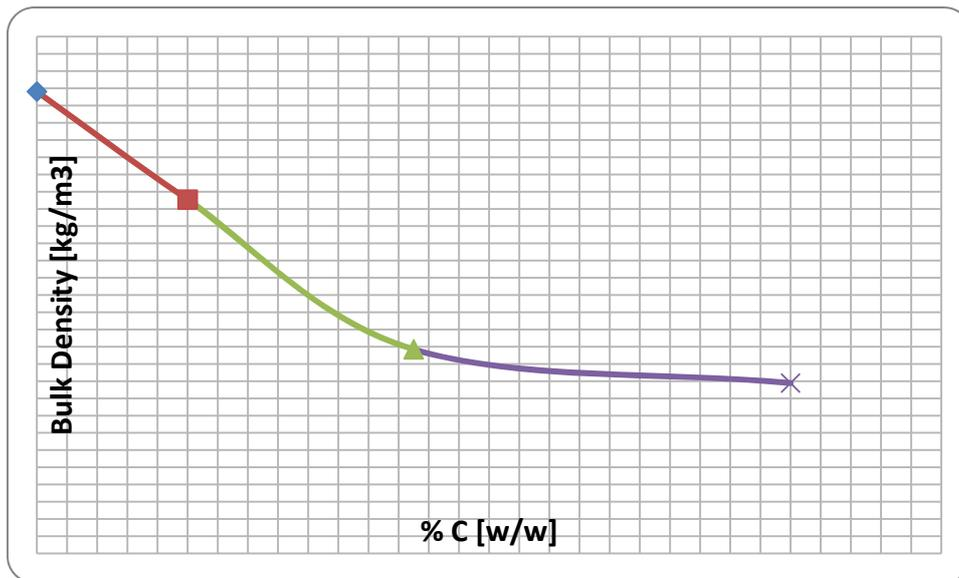
Figure 9. Bulk density of the self-reducing pellets as a function of the graphite concentration.
