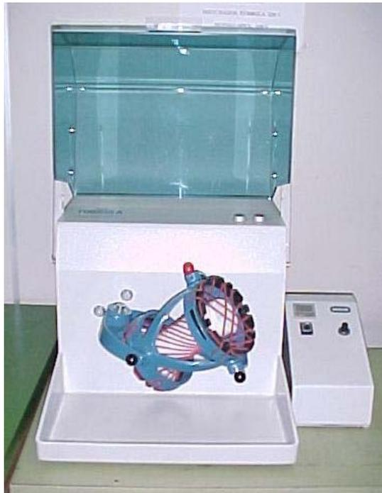
**Figure 2.** Turbula mixer to homogenize the mixture.
