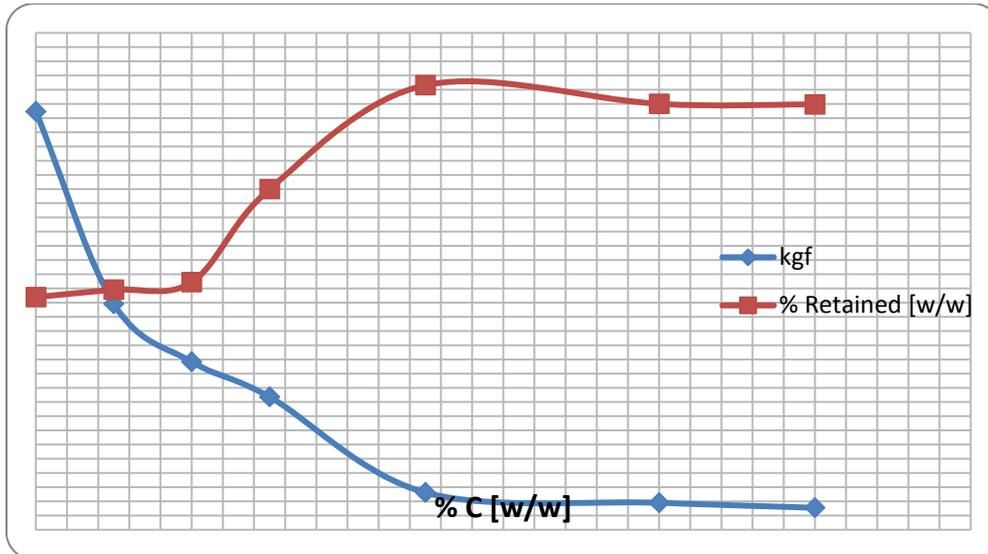
Figure 8. Cold compressive strength and abrasion resistance as a function of graphite concentration.
