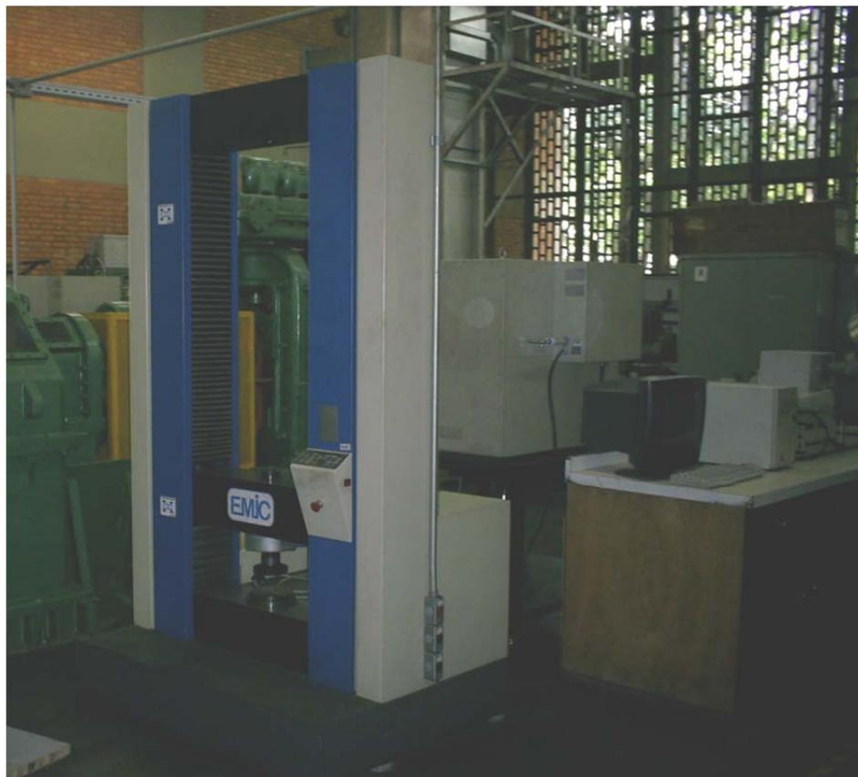
**Figure 3.** EMIC Press for compression tests, with capacity up to 30 tons.
