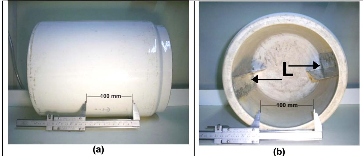
**Figure 4.** View (a) side and (b) front jar of porcelain, showing the L lifters.
