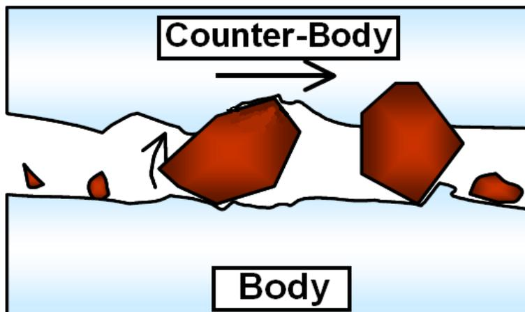
**Figure 1.** The schematic representation of wear three abrasive bodies <sup>[3]</sup>.
