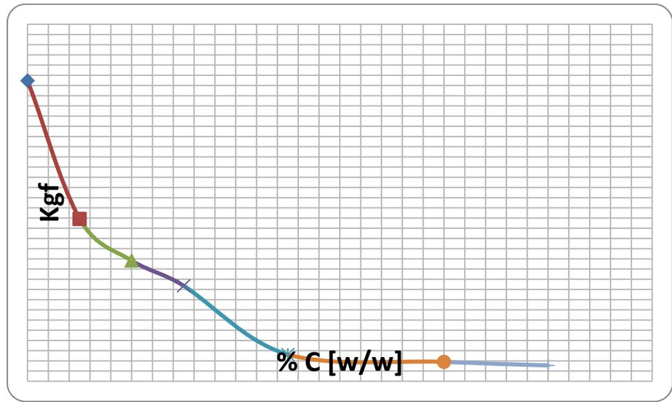
**Figure 6.** Compressive strength as a function of the graphite concentration.
