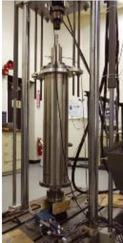
Figure 3: NIST test vessel for pressurized hydrogen gas
