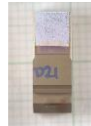
Fracture toughness at 3000 psi hydrogen pressure
