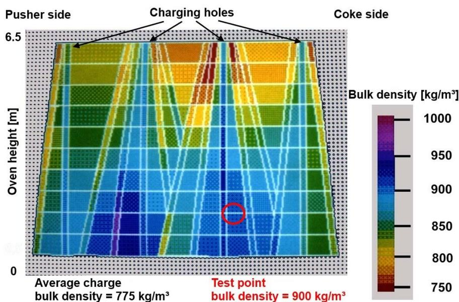
Figure 12. Bulk density distribution in a 6m coke oven.
