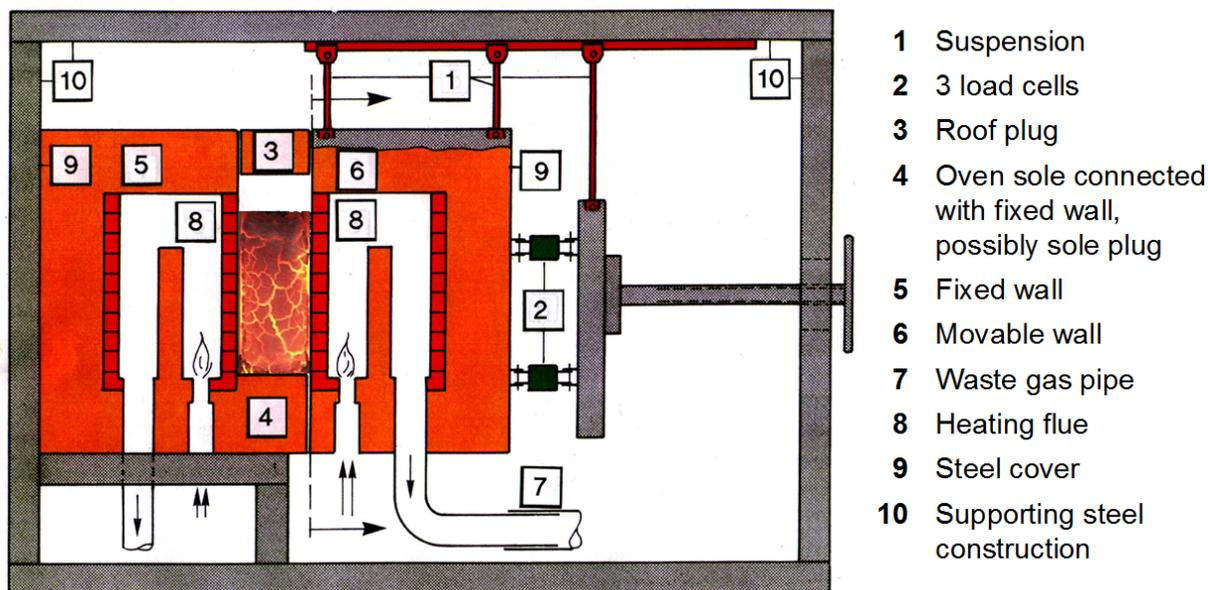
**Figure 1.** Semi-industrial carbonization test oven with movable wall.
