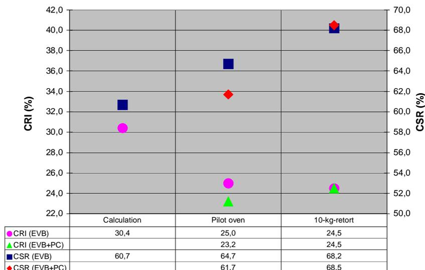
**Figure 10.** Comparison of calculated and measured CRI and CSR values for the Elk Valley Blend (EVB) without and with pet coke addition.
