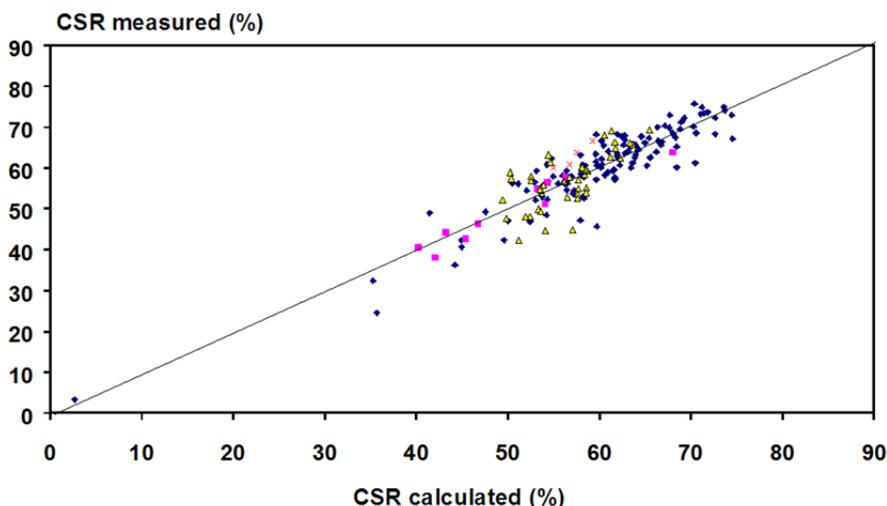
**Figure 8.** Comparison of measured and calculated CSR values.
