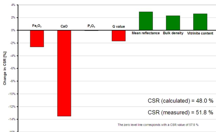
Figure 6. Influences of different coal characteristics on CSR of coal R2.
