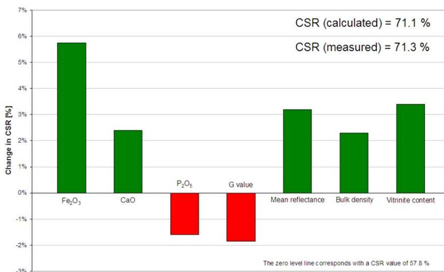
Figure 4. Influences of different coal characteristics on CSR of coal R1.
