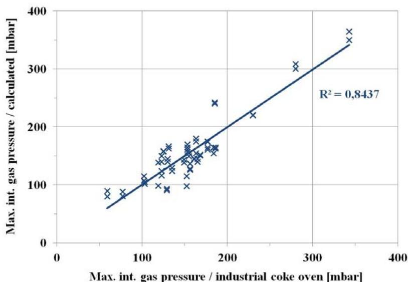
**Figure 14.** Comparison of measured and calculated max. int. gas pressure.
