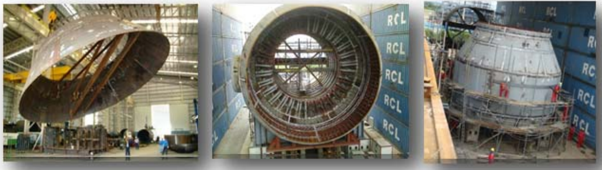
Figure 5. Examples of large vessel shells manufactured within Danieli Thailand.
