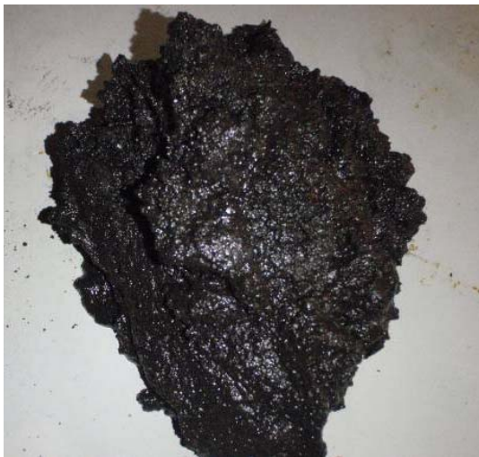
Figure 2: Oily sludge (8%TOC 19%H 2 O) and PLD product (Residual TOC < 0,1%)
