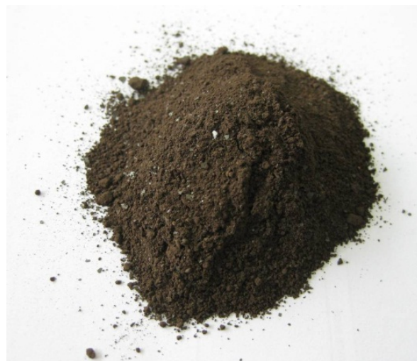
Figure 2: Oily sludge (8%TOC 19%H 2 O) and PLD product (Residual TOC < 0,1%)
