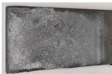
Fig. 4. Photo of the cathode employed in the EED lab-scale tests showing a up 90% Sb-Recovery.
