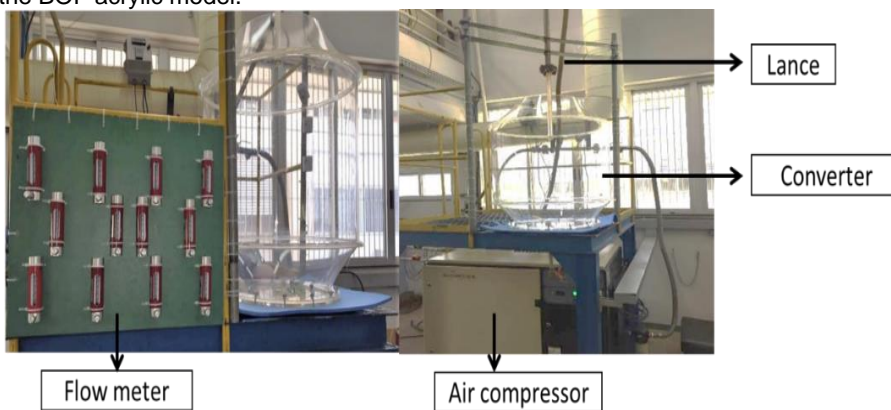
Figure 2: BOF cold model structure in LaSiP.
