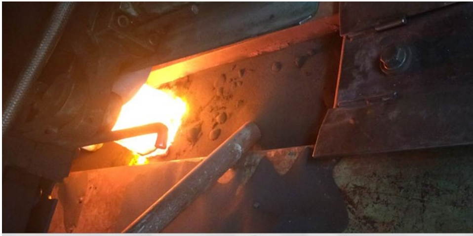
Figure 13. Agglomerate powder (spots) on the meniscus with fluorine – free
