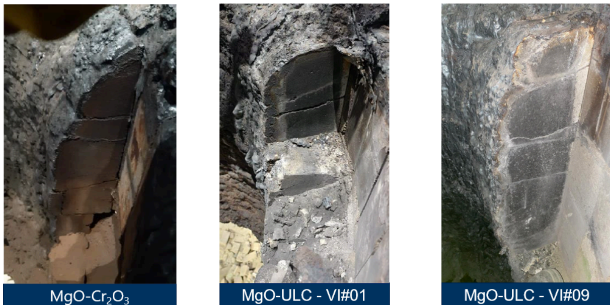
Figure 9. Comparison between the MgO and MgO-Cr 2 O 3 .
