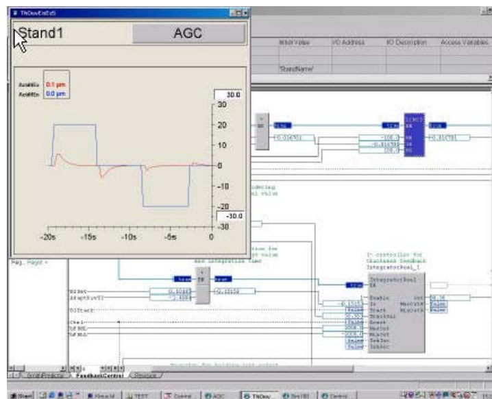
Figure 6. View of the Control Builder, Function plan representation acc. to IEC61131
