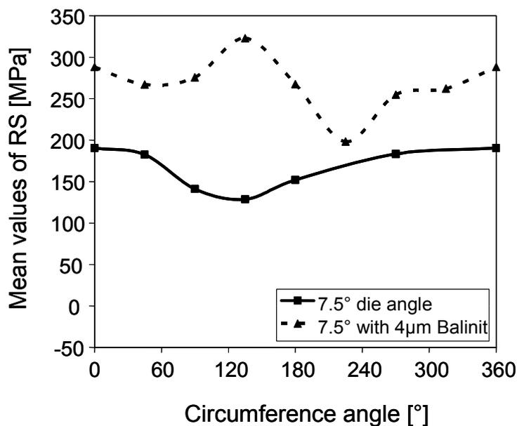
**Figure 8** - Mean values of residual stresses (RS) plotted against the circumference angle. Values at 360° were set to be equal to 0°.
