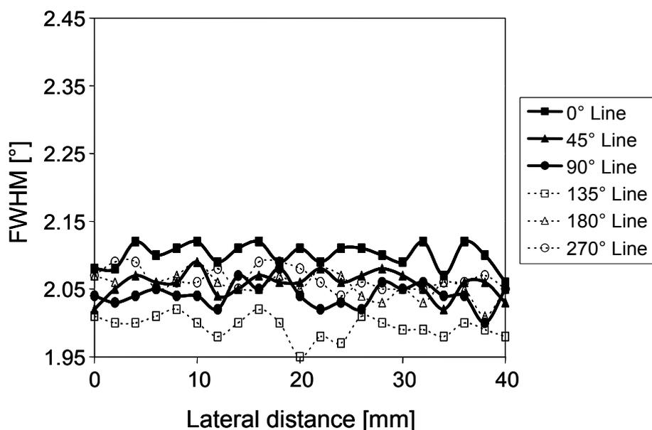
**Figure 10** - Full width at half maximum of {211} diffraction lines of plotted against axial distance along different lines around the circumference of a drawn bar after removal of a 50µm thick surface layer (7,5° semi-die angle).
