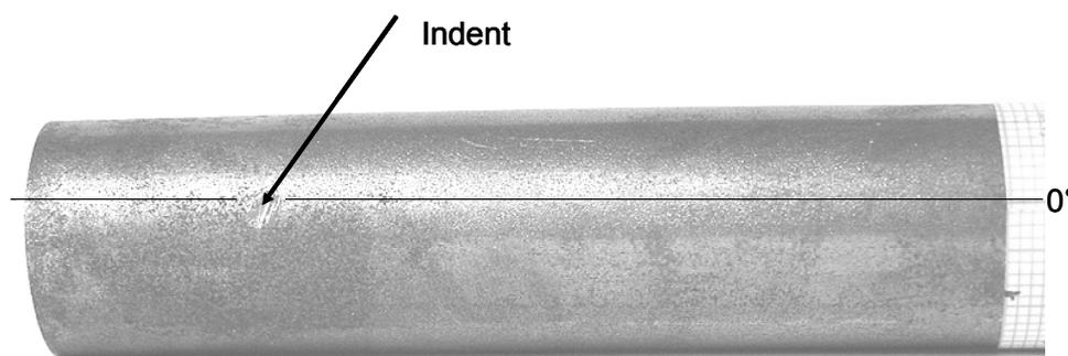
**Figure 7** - Sample of results in Figure 7, indent within at the 0° analysis line.
