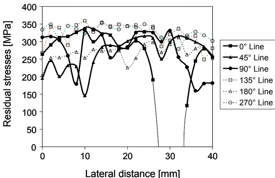
**Figure 6** - Residual stresses plotted against axial distance along different lines around the circumference of a drawn bar (TiCN coated tool with 7,5° semi-die angle).
