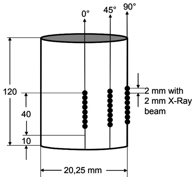
Figure 3 - Measurement procedure.
