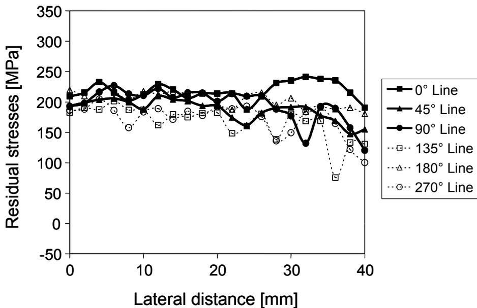
**Figure 9** - Residual stresses plotted against axial distance along different lines around the circumference of a drawn bar after removal of a surface layer of 50µm in thickness (7,5° semi-die angle).
