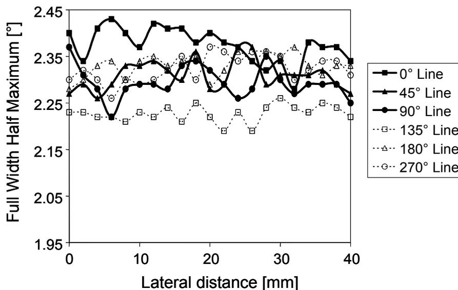
**Figure 5** - Full width at half maximum of {211} diffraction lines plotted against axial distance along different lines positioned around the circumference of a drawn bar (7,5° semi-die angle)
