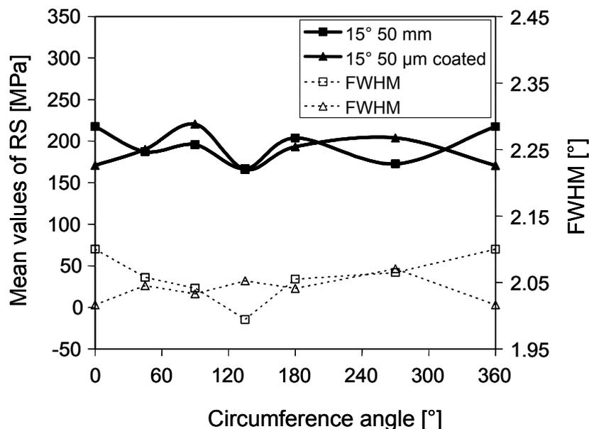
**Figure 11** - Mean values of residual stresses (RS) and FWHM plotted against the circumference angle after a surface layer removal of 50  $\mu\text{m}$  for the uncoated and the coated tool. Values at  $360^\circ$  were set to be equal to  $0^\circ$ .
