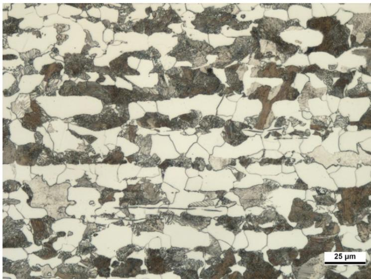
**Figure 2** - Longitudinal cross section of the investigated material, Nital 2%.
