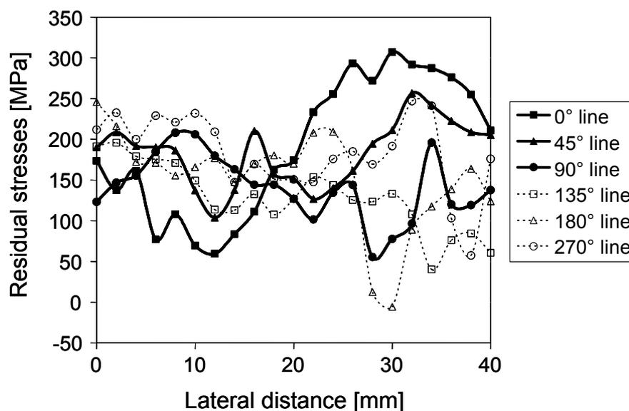
**Figure 4** - Residual stresses plotted against axial distance along different lines around the circumference of a drawn bar (7,5° semi-die angle)
