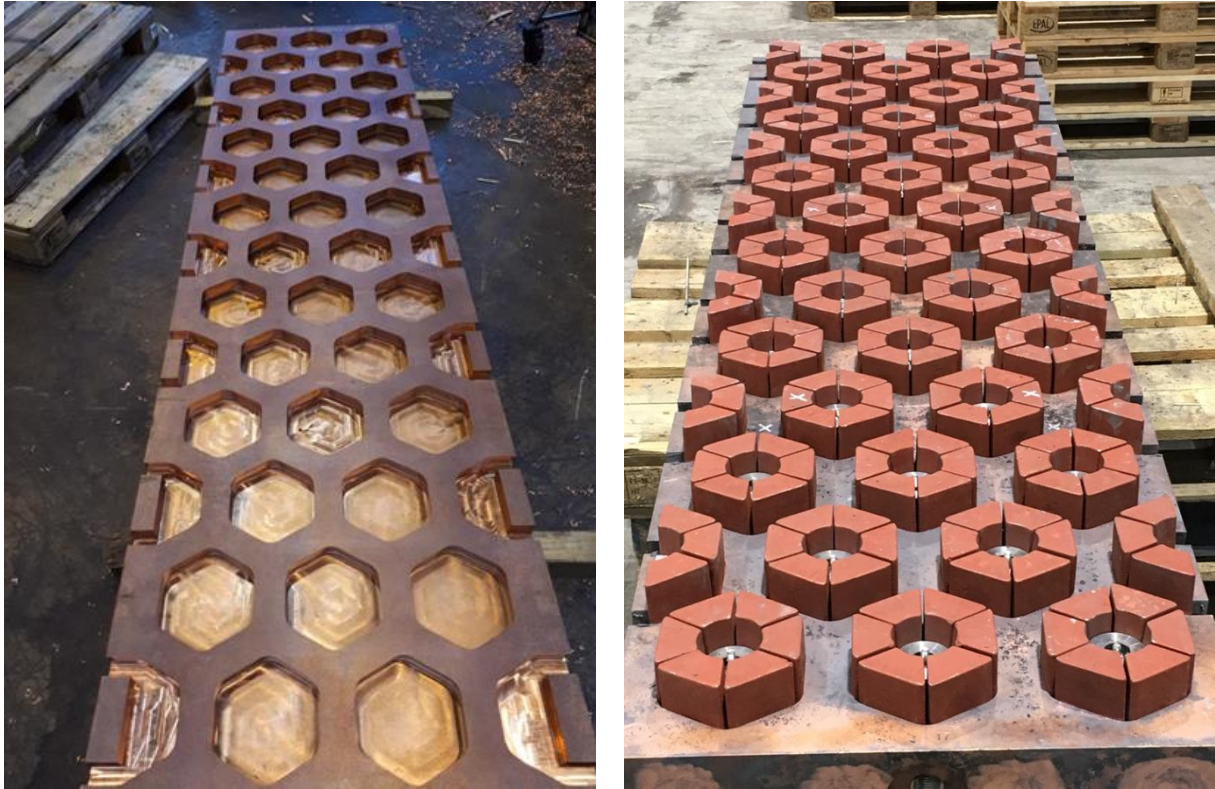
Figure 6. Honeycomb Stave Manufacture
