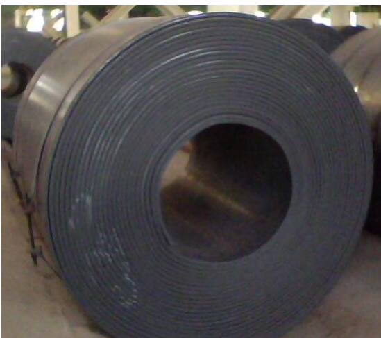
Figure 14. X80 coil of 21.4mm in thickness
