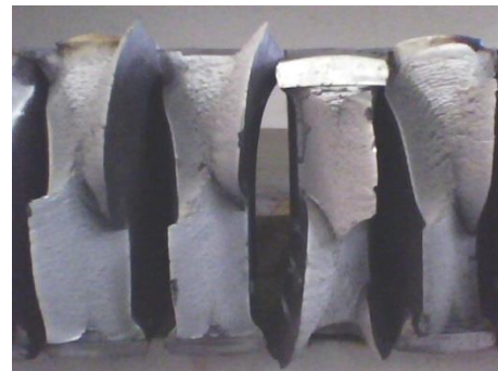
Figure 18. fracture morphology of 21.4mm X80 coil
