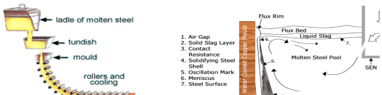
Figure 1. Schematic drawings of (a) the continuous casting process (4) and (b) the various slag layers formed in the mould (5)
