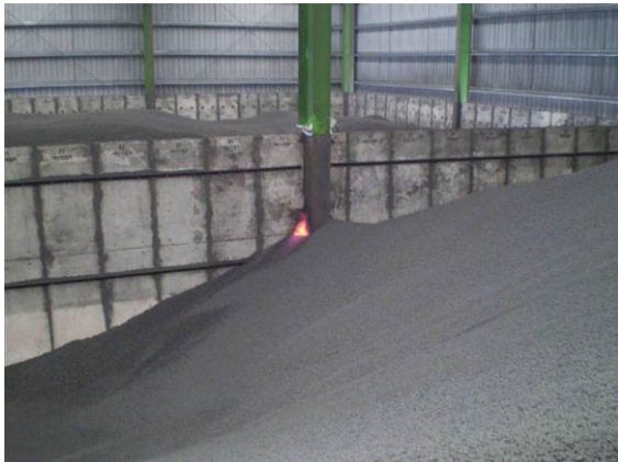
Figure 3. DRI burning in warehouse.
