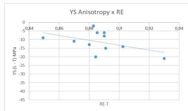
Figure 8: Yield strength anisotropy variation as a function of the YS/TS ratio for alloy 2.
