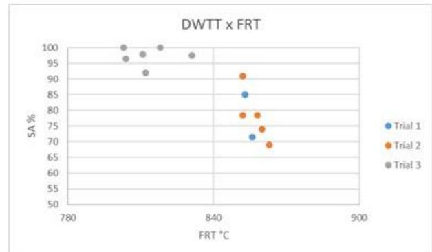
Figure 16: DWTT results for alloy 1.
