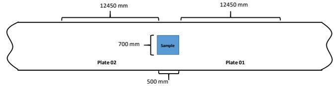
Figure 2: Sketch showing the sample location within the rolled unit.
