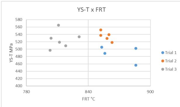
Figure 3: Transverse yield strength variation as a function of the FRT – Alloy 1.
