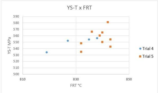
Figure 5: Transverse yield strength variation as a function of the FRT – Alloy 2.
