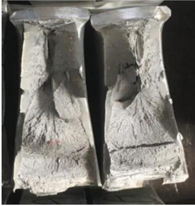
Figure 18: DWTT test piece surface showing inverse fracture.
