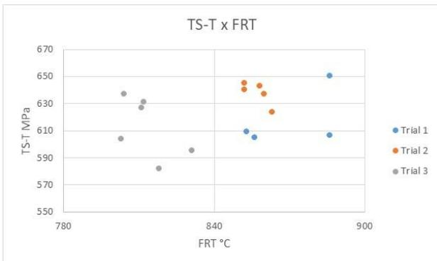
Figure 4: Transverse tensile strength variation as a function of the FRT – Alloy 1.
