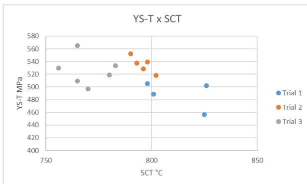
Figure 9: YS/TS ratio variation as a function of SCT for alloy 1.
