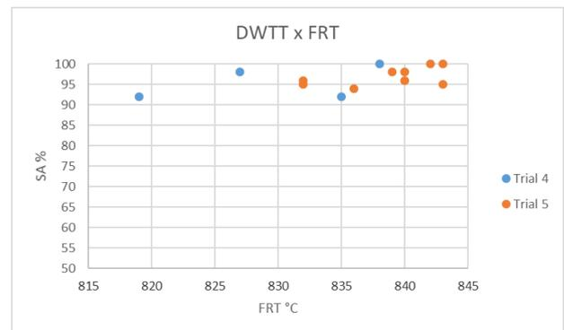
Figure 17: DWTT results for alloy 2.
