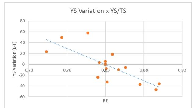
Figure 7: Yield strength anisotropy variation as a function of the YS/TS ratio for alloy 1.
