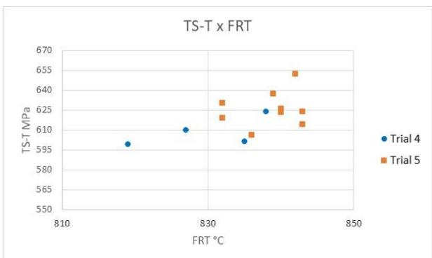
Figure 6: Transverse tensile strength variation as a function of the FRT – Alloy 2.
