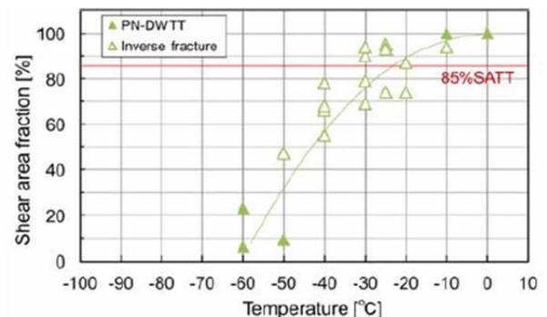
Figure 1: Comparison of shear area transition curve between PN-DWTT and pipe burst test [1].
