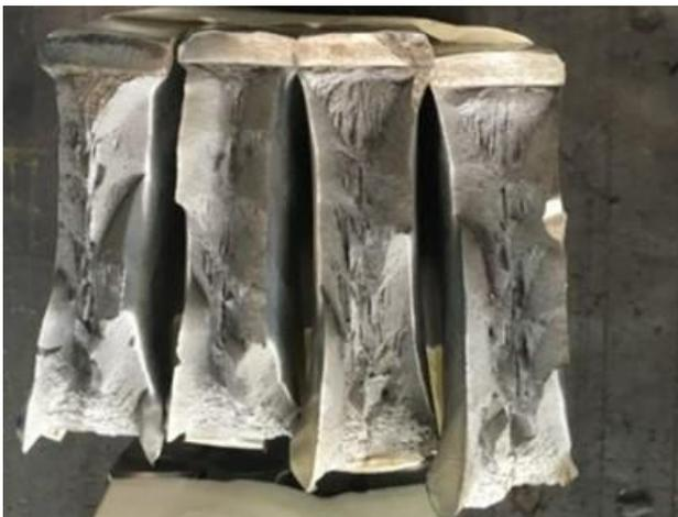
Figure 20: DWTT reduced specimen.
