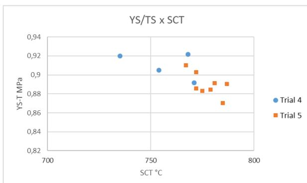
Figure 10: YS/TS ratio variation as a function of SCT for alloy 2.
