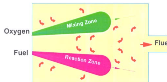
Figure 4: Schematic illustrating the Dilute Oxygen Combustion (DOC) concept.
