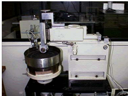
Figure 7: Rubber wear machine using asphaltic discs as counterfaces.
