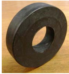
Figure 8: Counterbody used on the testing machine (diameter 80 mm, thickness 20 mm).
