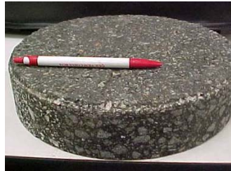
Figure 9: Counterface used on the testing machine (diameter 250 mm, thickness 50 mm).
