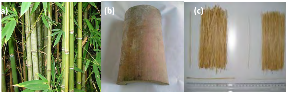
Figure 1. Bamboo trees (a), dried bamboo culm (b) and its fibers longitudinally stripped with different diameters (c).
