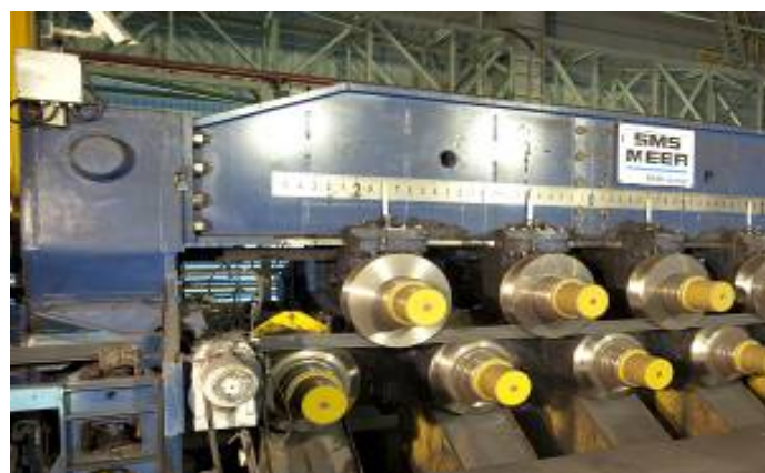
Figure 17. Roller straightening machine with adjustable pitch.
