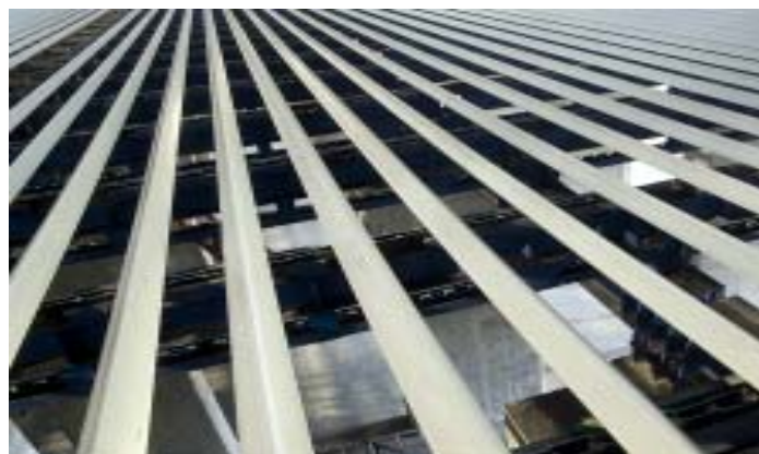
Figure 16. Equal Angles on the cooling bed.
