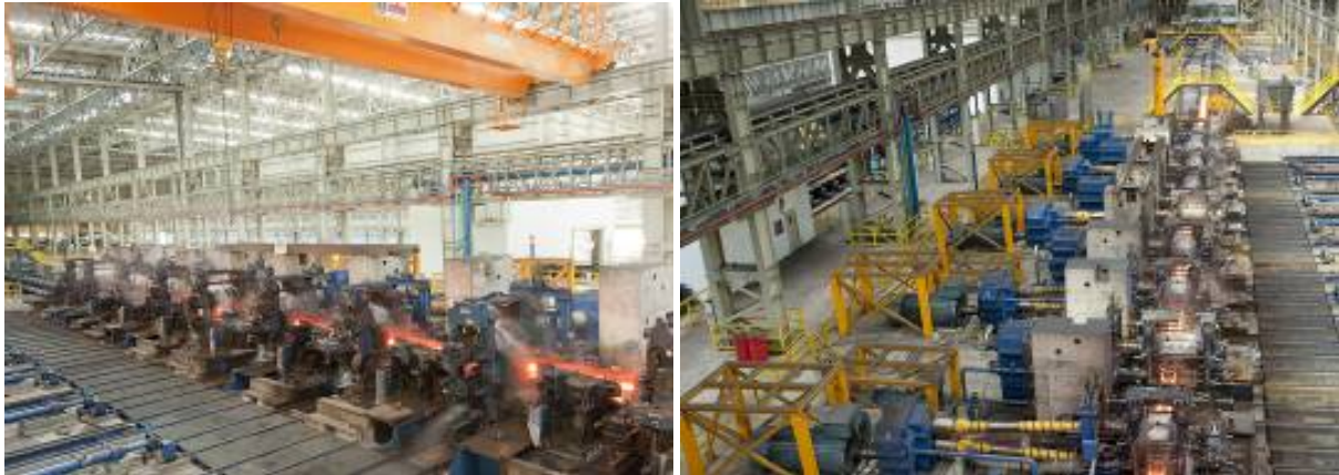
Figure 12. Finishing mill train (operator's side).
