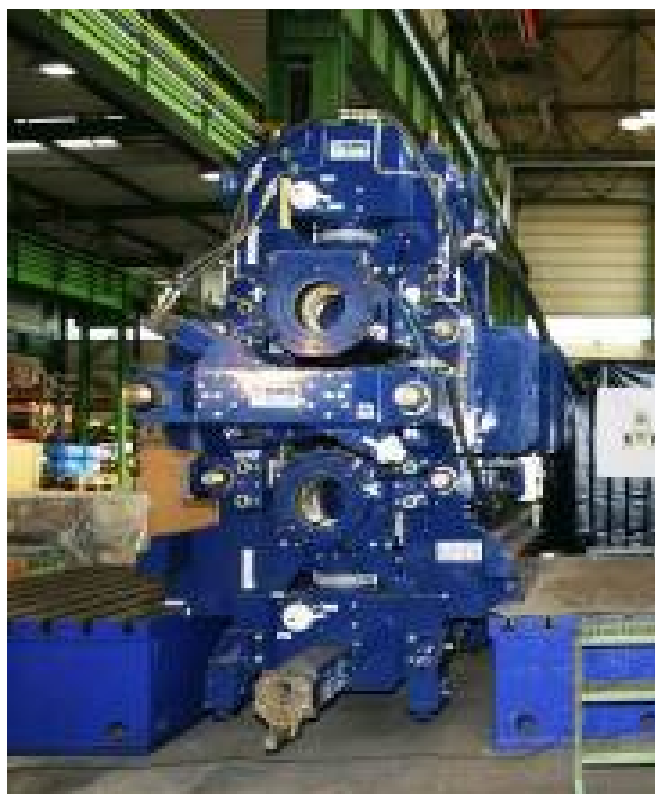
Figure 21. CS-stand in SMS Meer workshop for workshop test.
