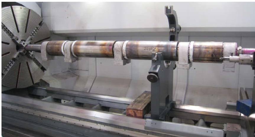
Figure 8. Machining of EcoStar roller for reuse.
