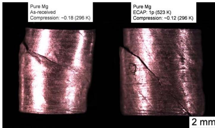
**Figure 4.** Appearance of the workpieces of the (left) as-received material and (right) material processed by ECAP after being tested in compression at room temperature up to failure.
