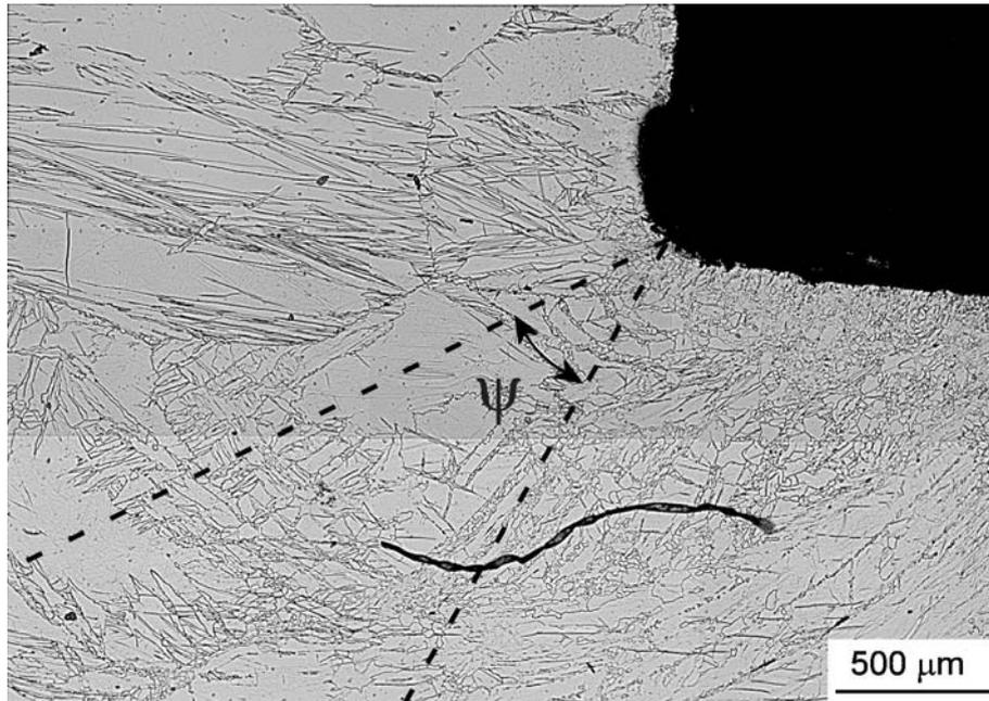
**Figure 2.** Grain structure in the region near the intersection between channels of the ECAP die. The dashed lines delineate the theoretical shearing zone.
