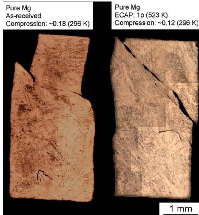
**Figura 5.** Grain structure along the longitudinal section of the workpieces of the (left) as-received material; and (right) material processed by ECAP after being tested in compression at room temperature up to failure.
