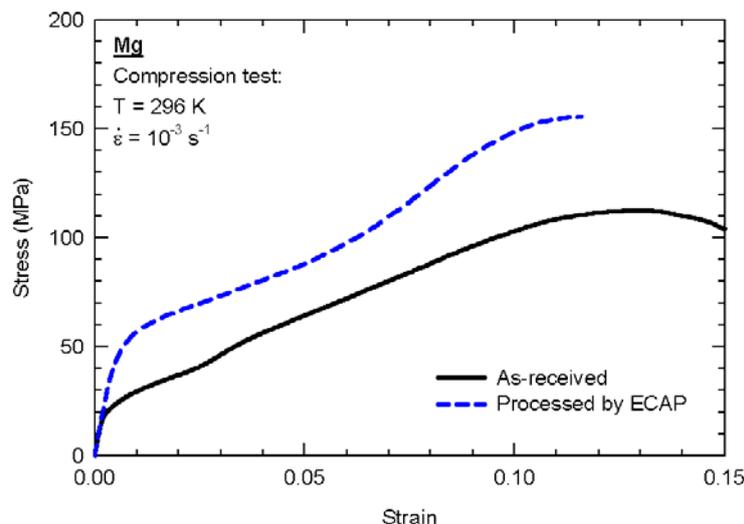
**Figure 3.** Stress vs. strain curves for the as-received material and the material processed by ECAP.
