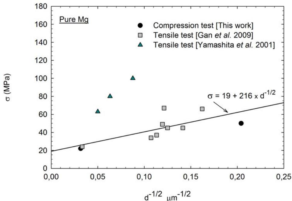
**Figure 7.** Flow stress as a function of the inverse of the square root of the grain size for pure magnesium processed by ECAP.
