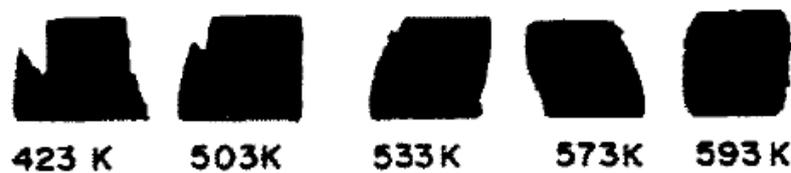
**Figure 1.** Appearance of the longitudinal section of samples of magnesium alloy after compression at different temperatures.<sup>(1)</sup>
