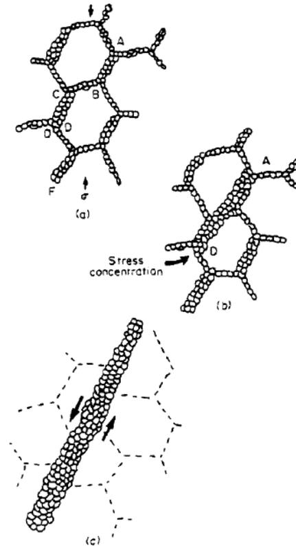
**Figure 6.** Illustration of the mechanism of formation of shearing bands during dynamic recrystallization of magnesium alloy proposed elsewhere.<sup>(1)</sup>
