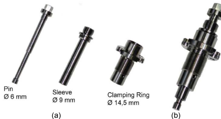
Figure 2. FSpW tool: (a) components (pin, sleeve and clamping ring); and (b) tool assembly.
