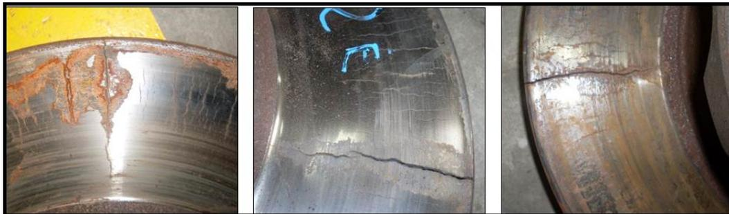
Figure 2. Cracks found on brake discs employed on heavy trucks.
