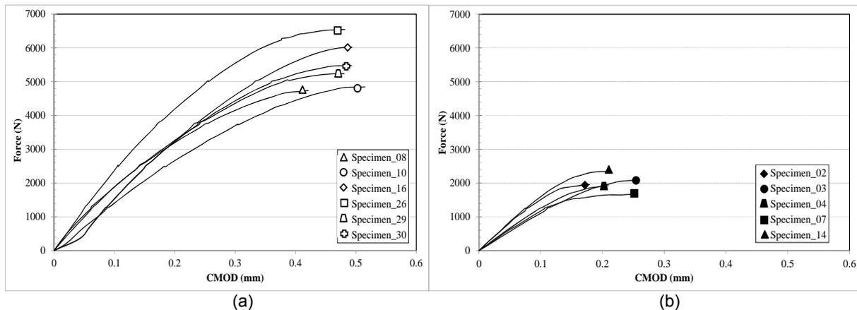
**Figure 8.** Load-displacement (CMOD) curves obtained from fracture mechanics tests carried out using the C(T) specimens of (a) as-cast material; and (b) heat treated material.
