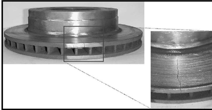
Figure 1. Cracks found on brake discs employed on Ford F-250 vehicles.<sup>(8)</sup>
