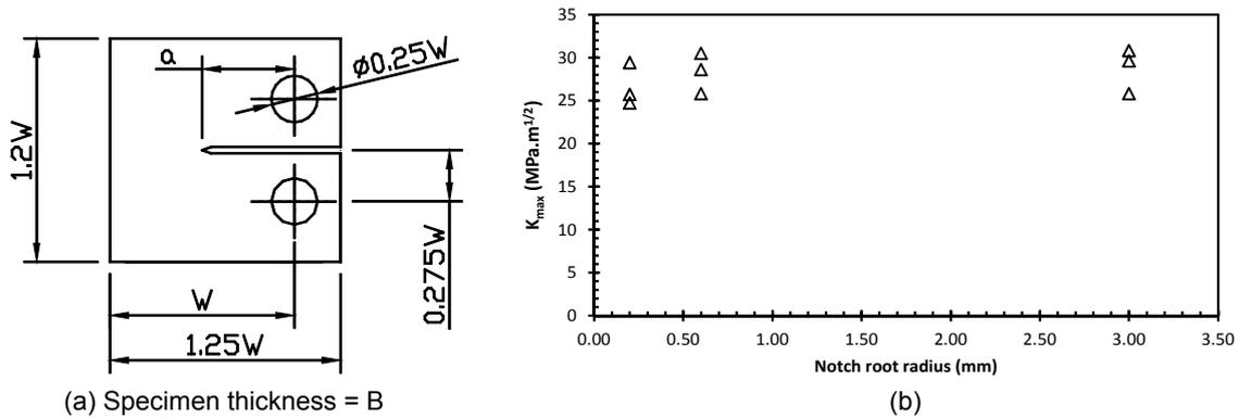
**Figure 3.** (a) C(T) fracture specimen; and (b) Fracture toughness ( $K_{max}$ ) evaluated for grey cast iron using SE(B) specimens with different notch root radius. Here,  $B = 15 \text{ mm}$ ,  $W = 30 \text{ mm}$  and  $a/W \approx 0.5$ .<sup>(12)</sup>
