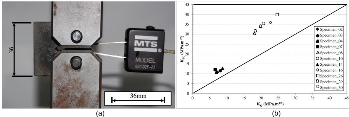
**Figure 9.** (a) Test scheme considering C(T) specimens; and (b) fracture toughness results considering  $K_{JC}$  and  $K_Q$  data. The solid line represents  $K_{JC} = K_Q$ .
