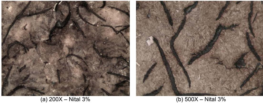
**Figure 4.** Micrographs for the studied grey cast iron consisting on A-type graphite in (a) ferritic-pearlitic matrix for the as-cast condition – graphite size 4; and (b) ferritic-pearlitic matrix with fine martensite and retained austenite for the heat-treated condition – graphite size between 4 and 5.
