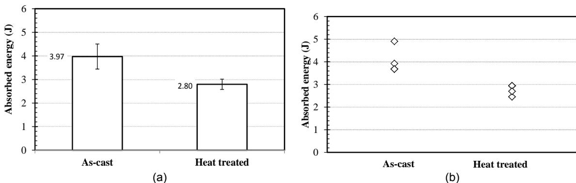
**Figure 5.** absorbed energy from Charpy tests for the as-cast and heat treated conditions.
