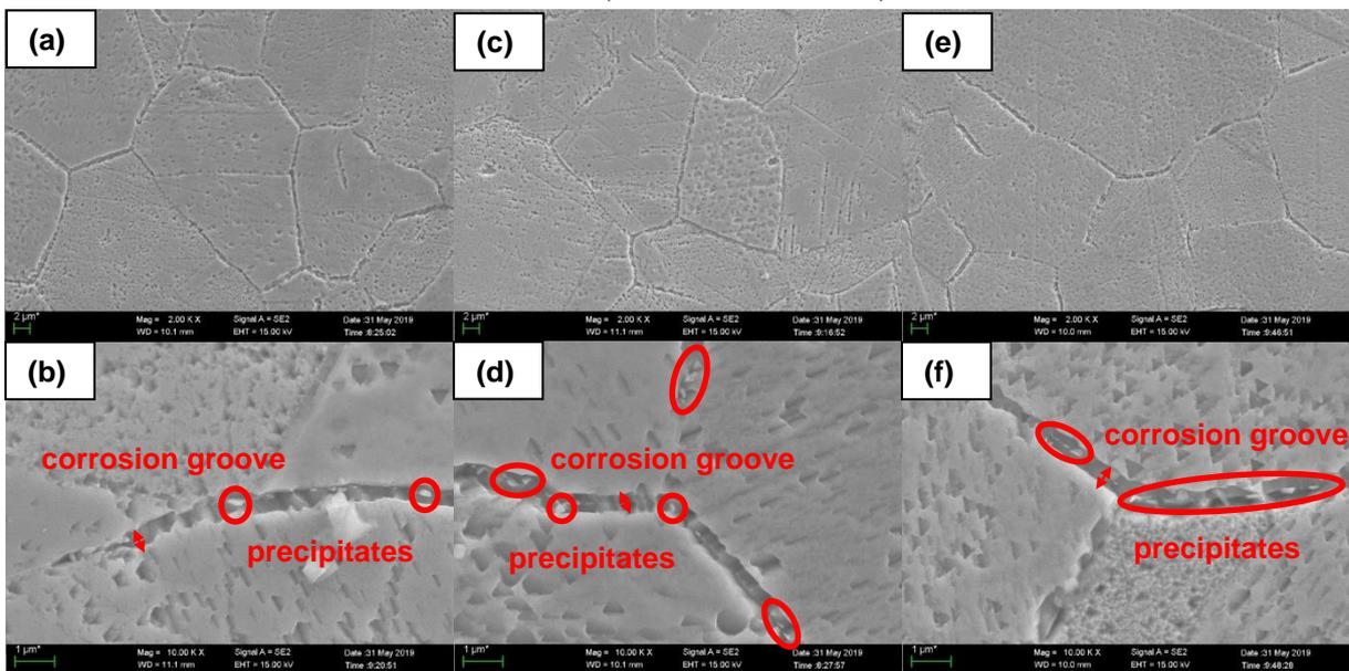
Fig. 3 SEM micrographs for samples of sensitization treatment at 500°C
