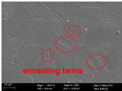
The microstructure of the standard solid solution treatment samples, observed by the scanning electron microscopy, was full austenitic structure which is shown in Fig. 2. It eliminates original precipitates that may have formed of the sample before any sensitization treatments. Investigation reveals equiaxial austenite grain intersected with annealing twins [11].
