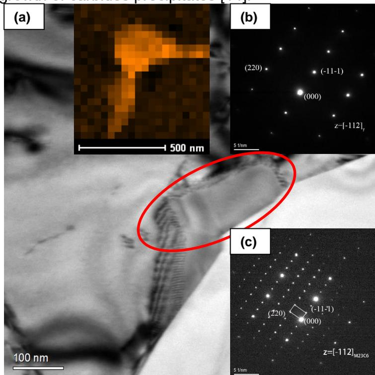
Fig. 10 TEM micrographs for the precipitate grows into the grain
