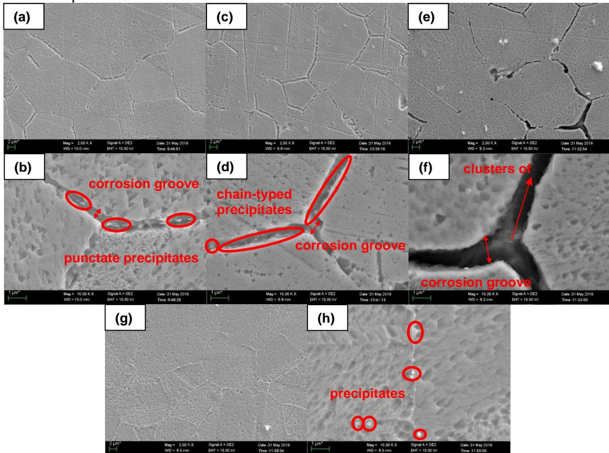
Fig. 4 SEM micrographs for samples of sensitization treatment at 15min
