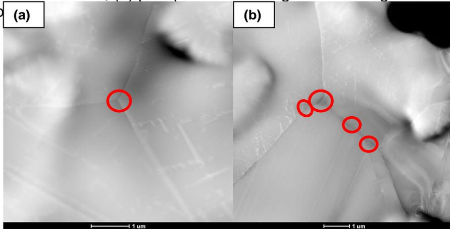
Fig. 9 TEM micrographs for the same sample (a) without precipitates; (b) precipitates
