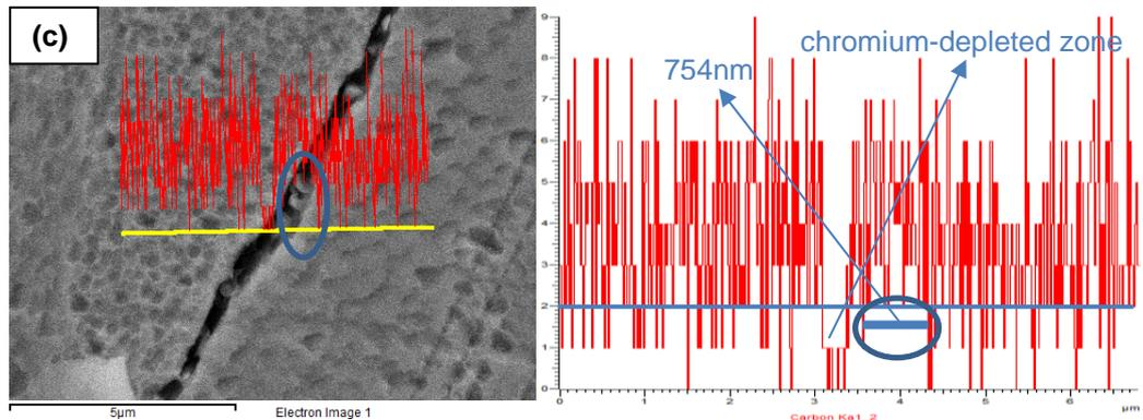
Fig. 7 linear scanning for sensitization at 5min (chromium) (a) 500°C; (b) 600°C; (c) 700°C
