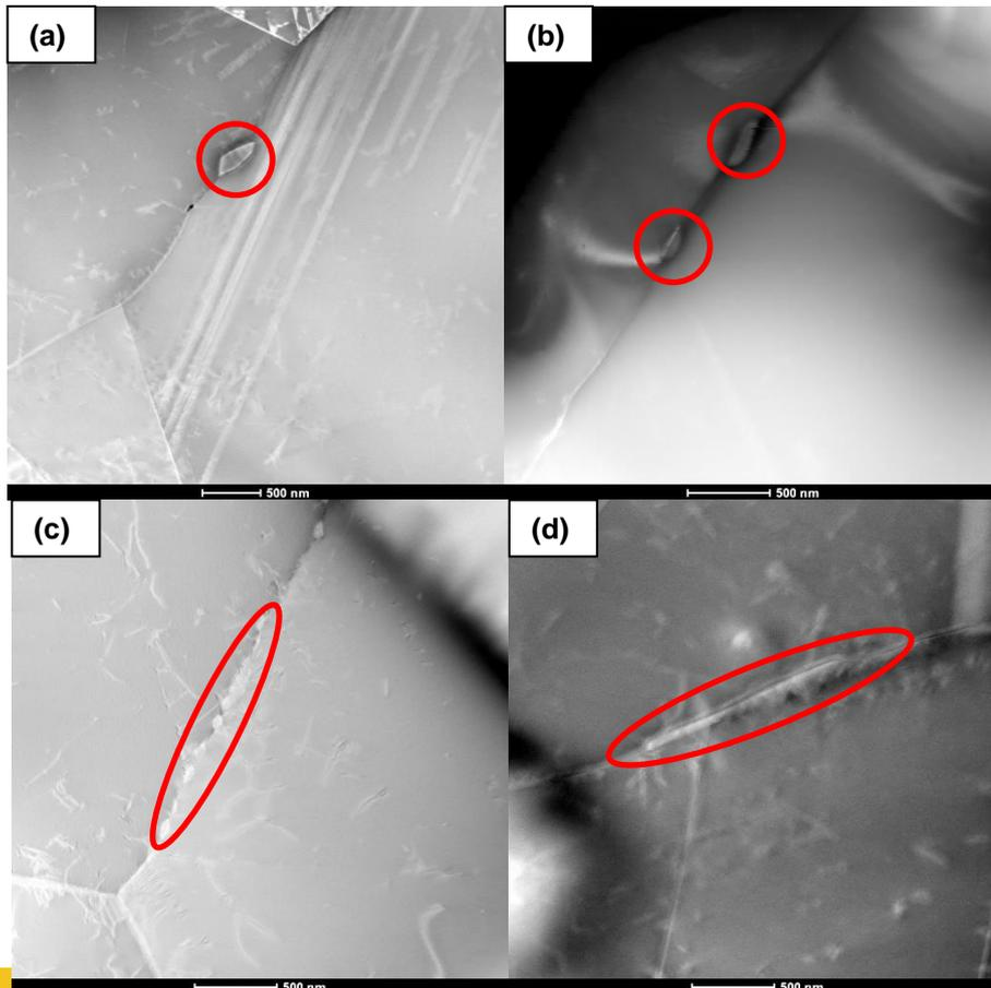
Fig. 8 TEM micrographs for samples of sensitization at 5min (a) 500°C; (b) 600°C; (c)700°C; (c)800°C
