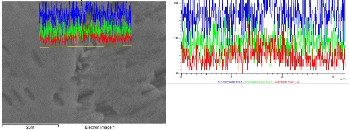
Fig. 6 linear scanning for samples of sensitization at 500°C for 5min
