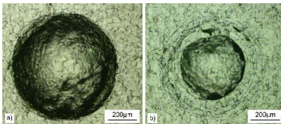
**Figure 5.** Brinell indentation on plasma nitrided samples of: (a) AISI 316 at 450°C, (b) AISI 316 at 500°C, (c) AISI 409 at 450°C and (d) AISI 409 at 500°C. 600Pa.
