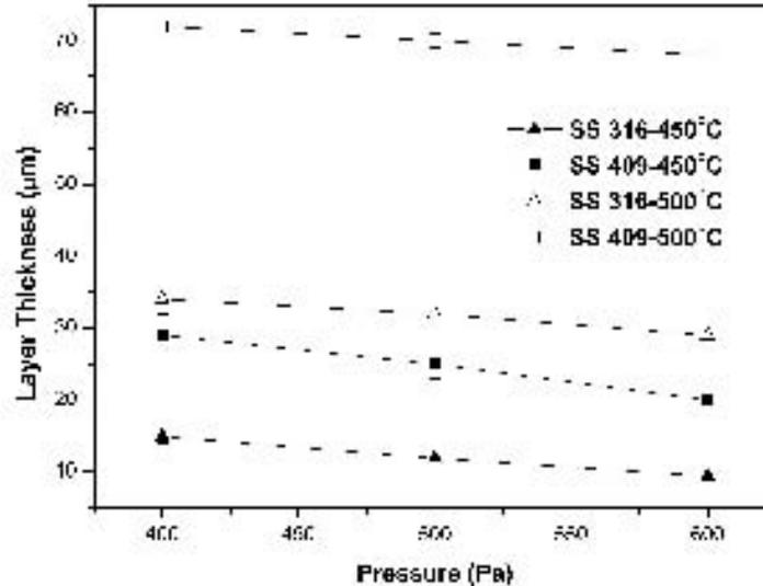
Figure 3. Layer thickness versus nitriding pressure, of plasma nitrided AISI 316 and 409.
