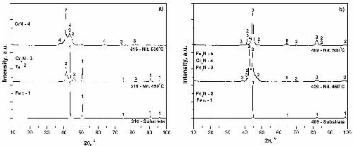
**Figure 2.** X-ray diffraction patterns of the non-nitrided and plasma nitrided samples of: (a) AISI 316; (b) AISI 409.
