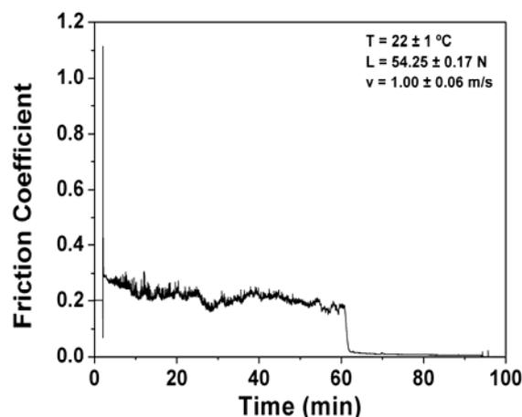
**Figure 2:** Si<sub>3</sub>N<sub>4</sub>-Al<sub>2</sub>O<sub>3</sub> friction coefficient lubricated with water. T - water temperature, L - applied load, v - sliding speed.
