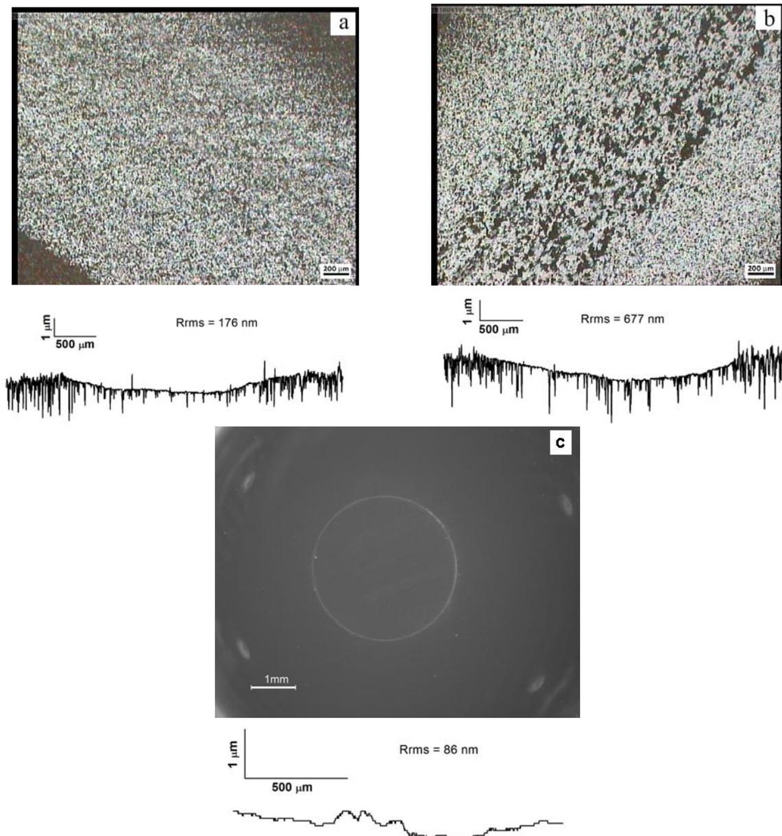
**Figure 4:** a and b disc wear tracks, c plateau on the ball with their respective roughness profiles.
