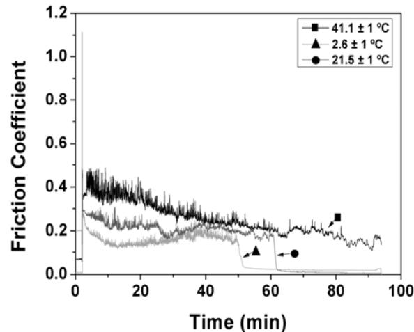
**Figure 3:** Friction coefficient versus sliding time, for  $\text{Si}_3\text{N}_4\text{-Al}_2\text{O}_3$ . Water. Constant temperature.
