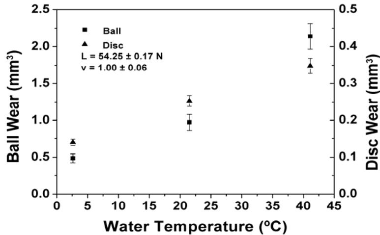
Figure 5: Wear volume versus water test temperature.
