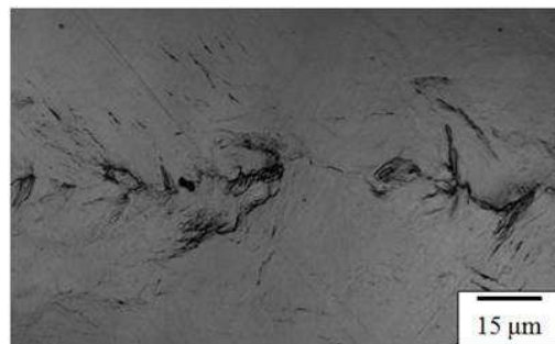
Figure 19. Localized slip in 10 MPa hydrogen gas, at 1 Hz, \Delta K = 17,5 \text{ MPa.m}^{1/2}
