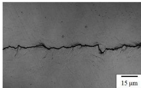
Figure 18. Localized slip in 45 MPa hydrogen gas, at 1 Hz, \Delta K = 17,5 \text{ MPa.m}^{1/2}
