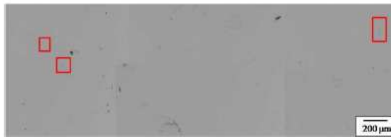
Figure 6. Inclusions observed on a polished surface of SNCM439 steel.
