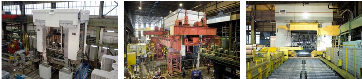
Figure 6. Pre-assembly of 160" millstand at SMS Siemag workshop (left), shifting to the final position at Aleris Aluminum Koblenz (middle), millstand in production (right).
