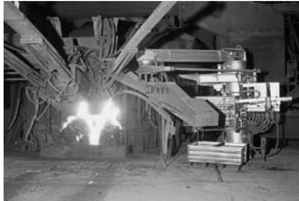
Figure 4. Using a manipulator to take a sample and temperature while foaming slag.
