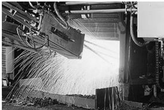
Figure 3. Slag Foaming using a Lance Manipulator
