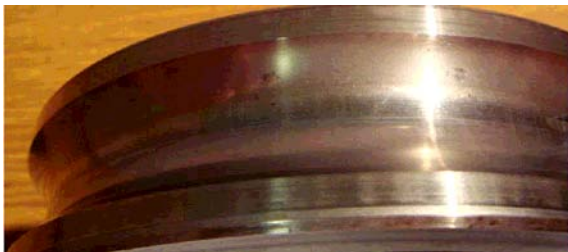
Figure 10. Bearing Inner race Pitting Failure
