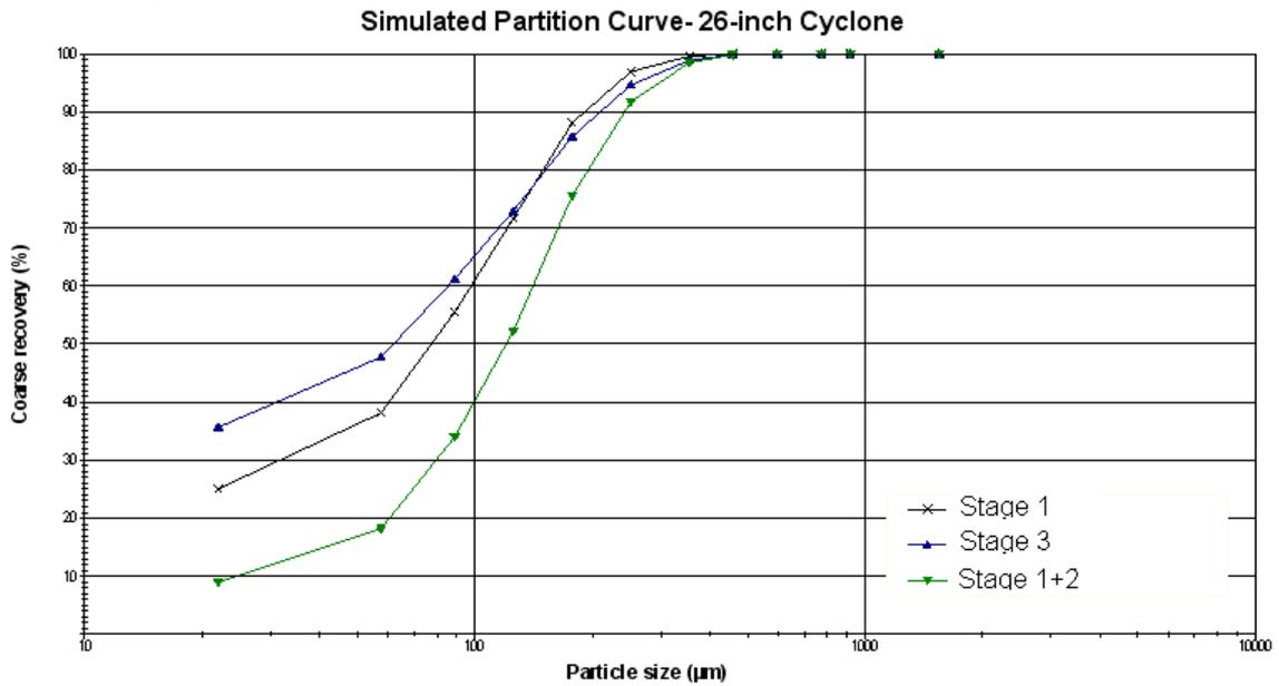
Figure 5: Simulated partition curves for a 26-inch cyclone
