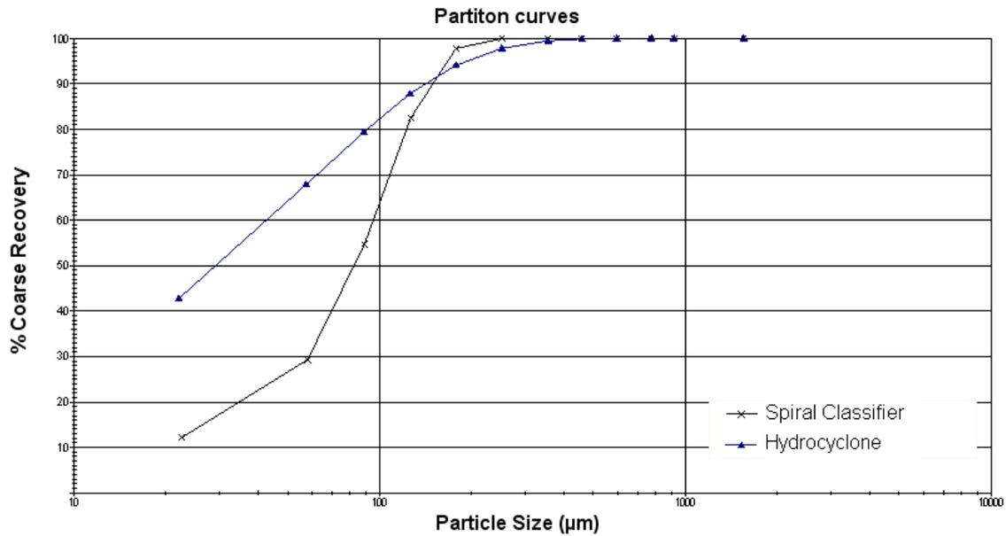
**Figure 3:** Partition curves of the spiral classifier and cyclone in the pilot test
