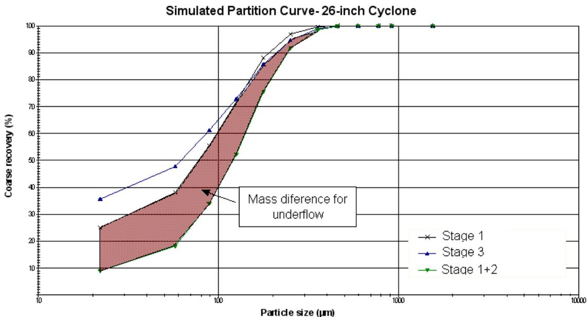
Figure 6: Comparison between the efficiency of a single classification stage and double classification stage for a 26-inch cyclone
