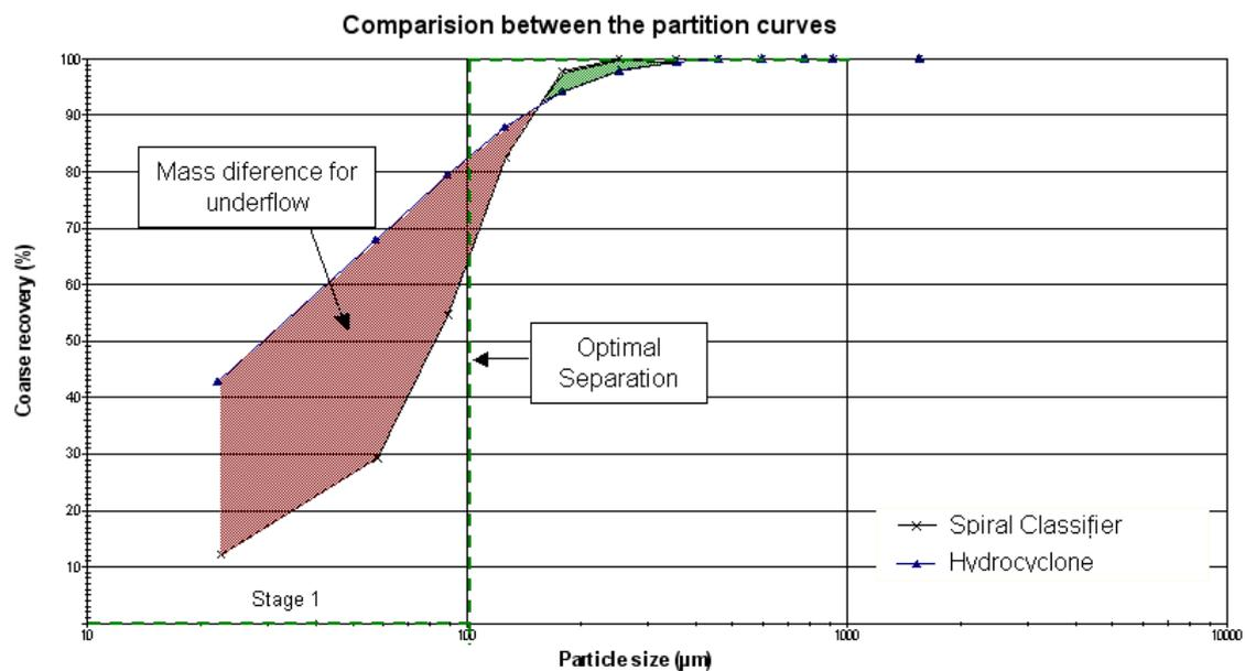
**Figure 4:** Comparison between the efficiency of the spiral classifier and cyclone in the pilot tests
