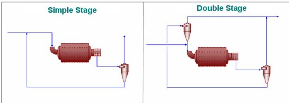
Figure 7: Simplified flow charts of the industrial circuits of simulated grinding
