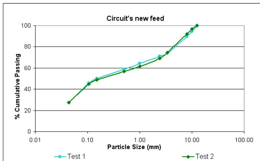
**Figure 2:** Granulometry of new feed in tests 1 and 2
