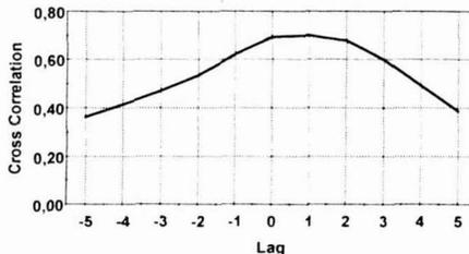
Figure 18. Cross correlation between top gas temperature and hot metal content for burden of sinter + KPBO.
