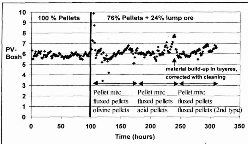
Figure 19. Reasonably stable PV-bosh for operations with 100% KPBO pellets and various mixed burdens of lump ore and pellets.
