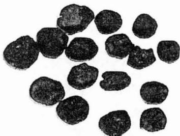
Figure 4. MPBO olivine pellets taken from the experimental blast furnace, with no evidence of swelling.
