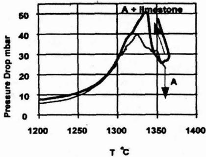
Figure 12. Laboratory meltdown test showing rapid carburisation and melting of a pellet at 1360°C, and a second test showing rapid increase in pressure drop upon the start of melting when there was a small amount of limestone added to the pellets.
