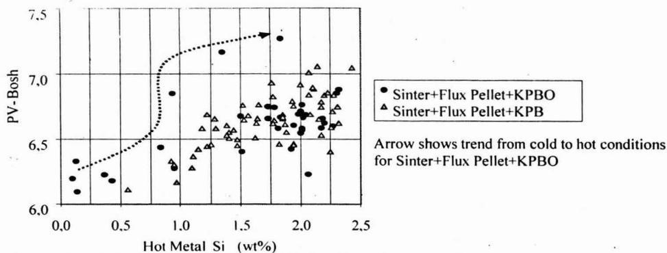
Figure 14. Relationships between PV-bosh and hot metal silicon content for sinter-pellet burdens showing a difference in behaviour between using acid and olivine pellets in the burden mix.
