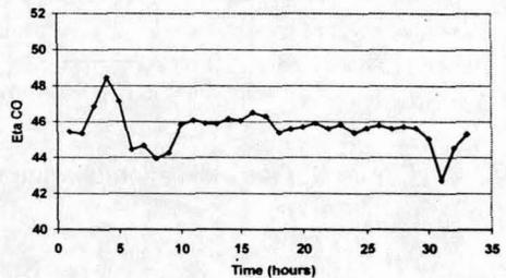
The difference in reducibility of LKAB pellets has not had a measurable effect on blast furnace performance, except perhaps that pellet C, with a high reducibility, had poor reduction strength and swelling which resulted in the unstable operation shown in Figure 5. When the pellet properties were good, such as for MBPO and Pellet E, the blast furnace fuel rates were not measurably different despite the great difference in reducibility.
