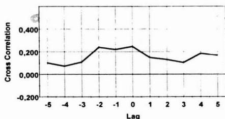
Figure 15. Cross correlation between top gas temperature and hot metal Si content burden of sinter + fluxed pellets + KPBO olivine pellets.
