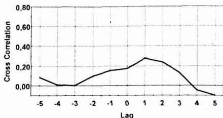
Figure 17. Cross correlation between temperature and hot metal Si content for burden of sinter + KPBO.
