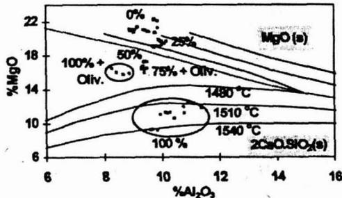
Figure 13. Primary phase fields shown for bosh slags formed with varying mixtures of pellets and lumpy olivine corresponding to the blast furnace tests in Figure 11. At 100% test pellets, without lumpy olivine addition, the primary phase field shown is dicalcium silicate with liquidus temperatures as high as 1540°C.
