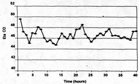
Figure 8. Variation in gas utilisation for commercial MPBO pellets in the blast furnace. In the furnace they exhibit very good reduction strength and little or no swelling, but in the laboratory test they do show a higher tendency to swell than Pellet E above.
