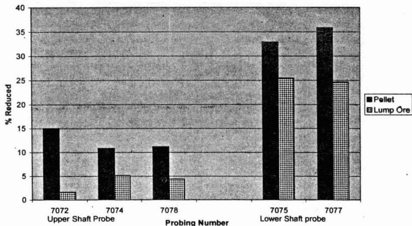
Figure 10. Comparison of the reduction of lump ore and pellets
