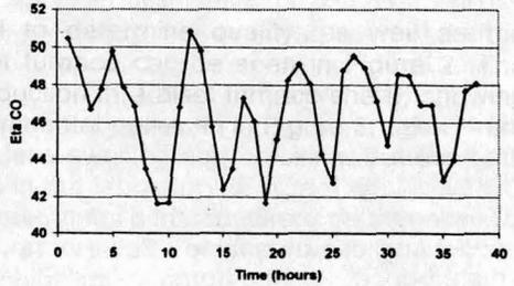
Figure 6. Variation in gas utilisation for experimental pellets, Pellets D in Figure 1, which showed reasonably good reduction strength and low swelling in the experimental blast furnace
