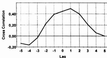
Figure 16. Cross correlation between top gas temperature and hot metal Si for content for burden of sinter + fluxed pellets + KPBO acid pellets.
