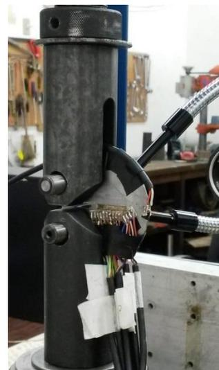
**Figure 7.** Assembly plane stress specimen,  $t = 2$  mm.
