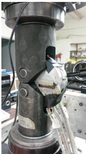
**Figure. 6.** Assembly plane strain specimen,  $t = 30$  mm
