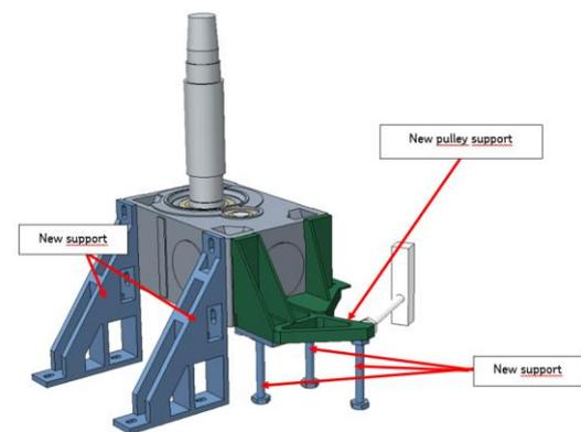
**Figure 8.** New supports applied to gearbox system.
