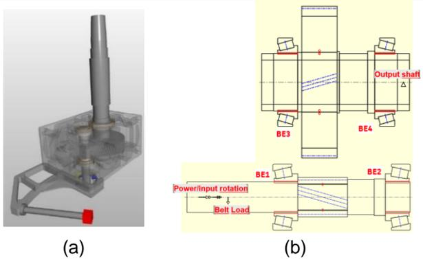
**Figure 9.** (a): CMS current condition model and (b): boundary conditions applied to gearbox system.
