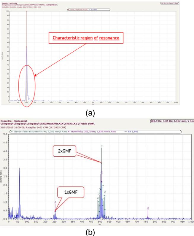
**Figure 2.** (a): vibration spectrum measured in the 11Z present characteristic of resonance and (b): vibration Spectrum measured in the 9X with misalignment event.
