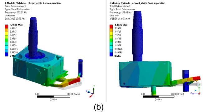
**Figure 6.** (a): Operational mode obtained by ODS in 109.4 Hz and (b): mode shape obtained numerically by FEM in 103.01 Hz.
