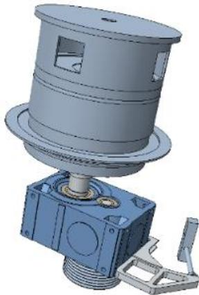
**Figure 4.** Gearbox System (gearbox, belt support, pulleys and drum).
