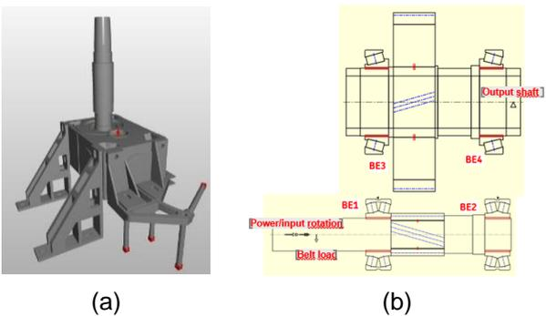
**Figure 10.** (a): CMS structural modifications condition model and (b): Proposal modification structural condition and new bearing arrangement (SRB).
