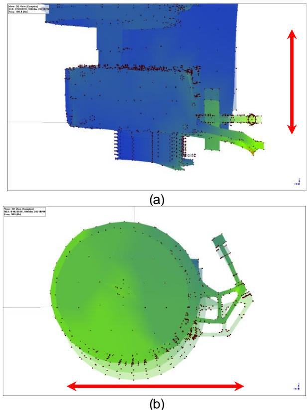
**Figure 3.** (a) and (b): Operational modes obtained by ODS in 109 Hz and 500 Hz frequencies highlighting the vertical and horizontal displacement, respectively.
