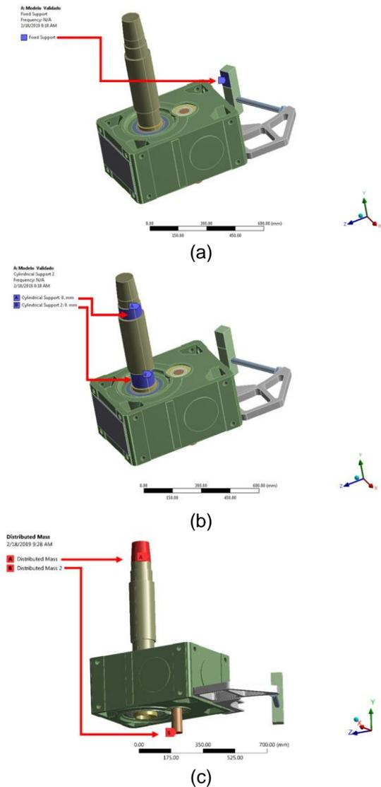
**Figure 6.** (a-c): Boundary Conditions applied to frame gearbox system.
