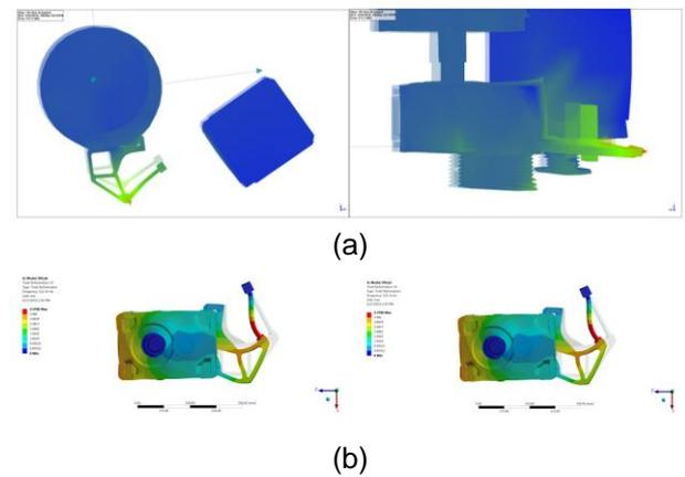
**Figure 7.** (a): Operational mode obtained by ODS in 511 Hz and (b): mode shape obtained numerically by FEM in 522 Hz.
