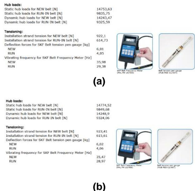
**Figure 14.** (a): Tension applied to SPB2650XP and (b): PHG XPB2650
