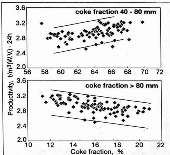
Fig. 18 The effect of coke properties on BF-2 performance at Rautaruukki Steel (1996 - 1998)
