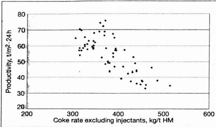
**Fig. 11 Coke rate versus productivity for W. European blast furnaces in 2000**
