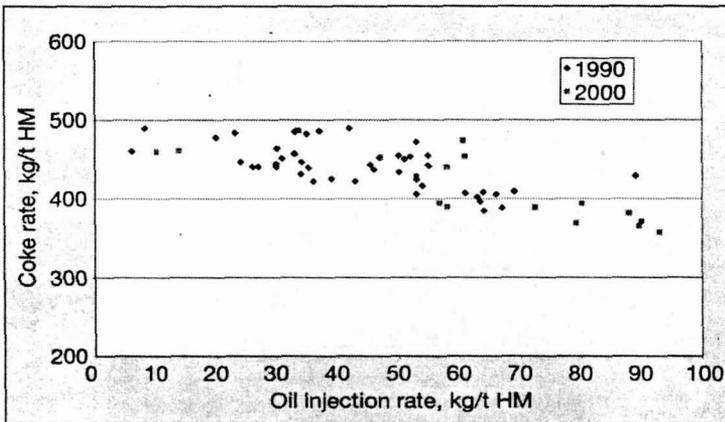
**Fig. 10 Coke rate versus oil rate for W. European blast furnaces**
