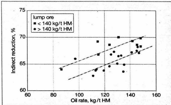
Fig. 17 Influence of lump ore ratio on the indirect reduction at HKM
