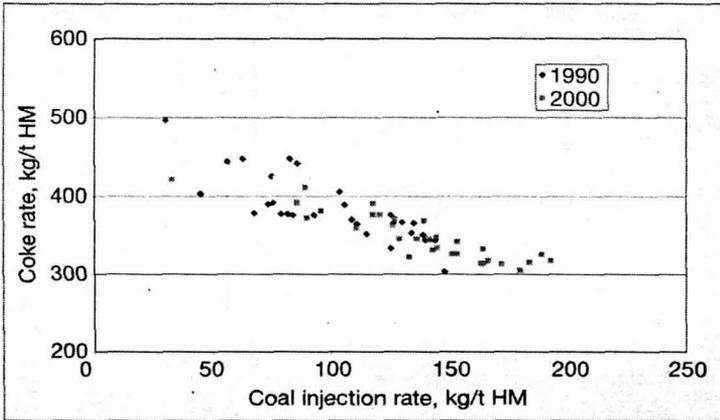
**Fig. 9 Coke rate versus coal rate for W. European blast furnaces**
