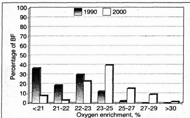
**Fig. 4 Comparison of oxygen enrichment in Western European BF in 1990 and 2000**
