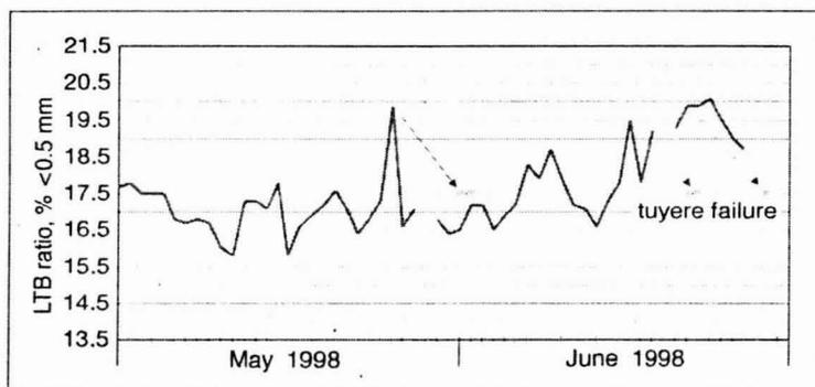
Fig. 16 Influence of sinter low temperature degradation on tuyere failures, Sidmar BF-B
