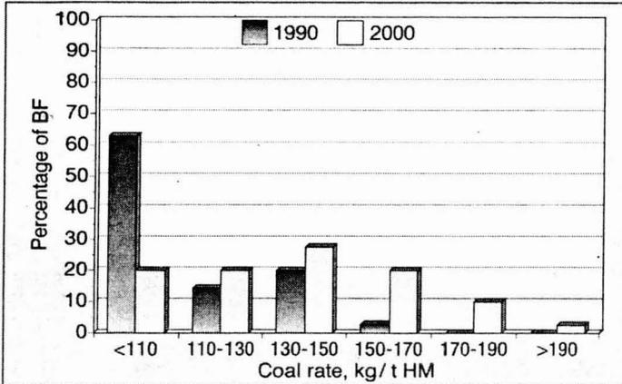
**Fig. 8 Comparison of BF coal injection rates in Western Europe in 1990 and 2000**
