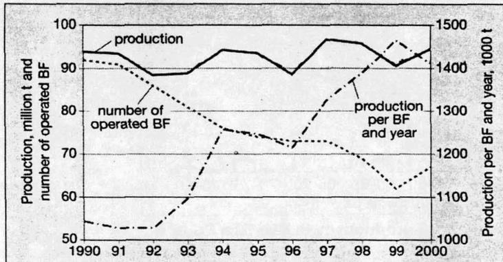
Fig. 1 Evolution of hot metal production in Western Europe, number of operated blast furnaces (BF) and production per BF and year
