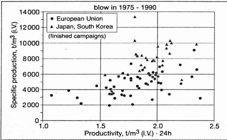
Fig. 24 Effect of productivity on specific production during a campaign
