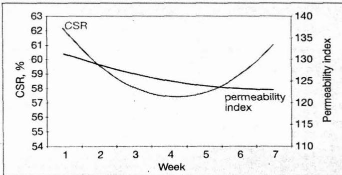
Fig. 22 Evolution of CSR (weekly values) and blast furnace permeability
