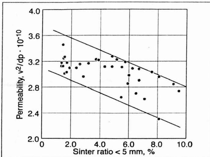
Fig. 15 Influence of sinter fines on the permeability, HKM BF-B
