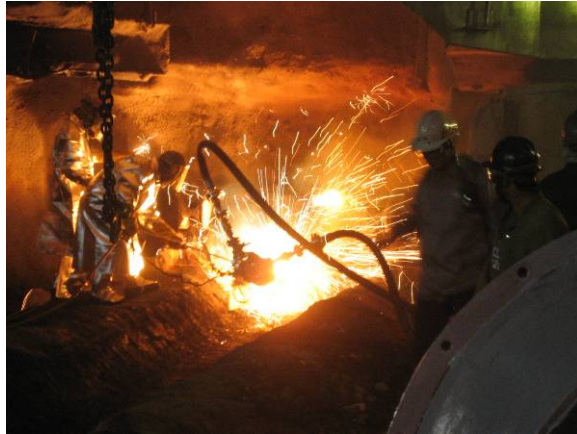
Figure 11 Cutting an oxy–fuel lance
