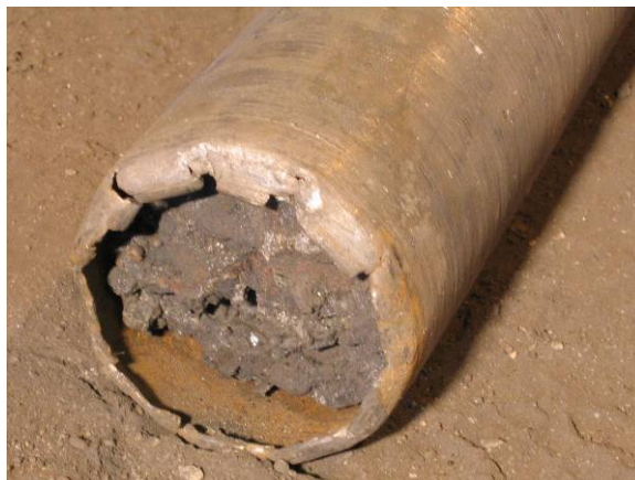
Figure 5 Damaged core drill: substantial amounts of solidified iron in hearth
