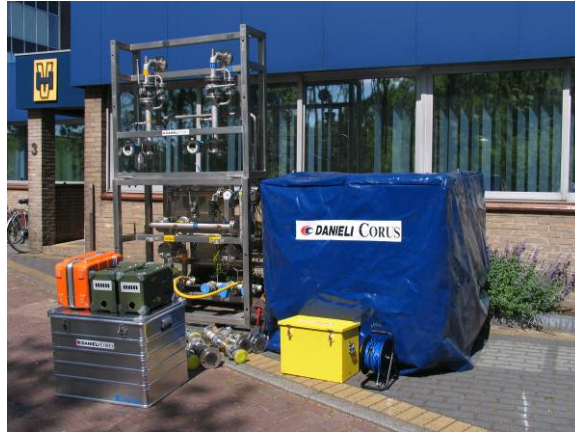
Figure 3 Oxy-fuel recovery equipment "ready to go"
