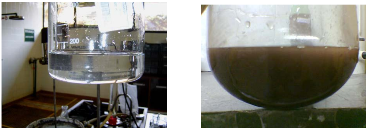
Figure 8: Filtrate clarity - Ceramec® filter (left) and RVDF (right)
