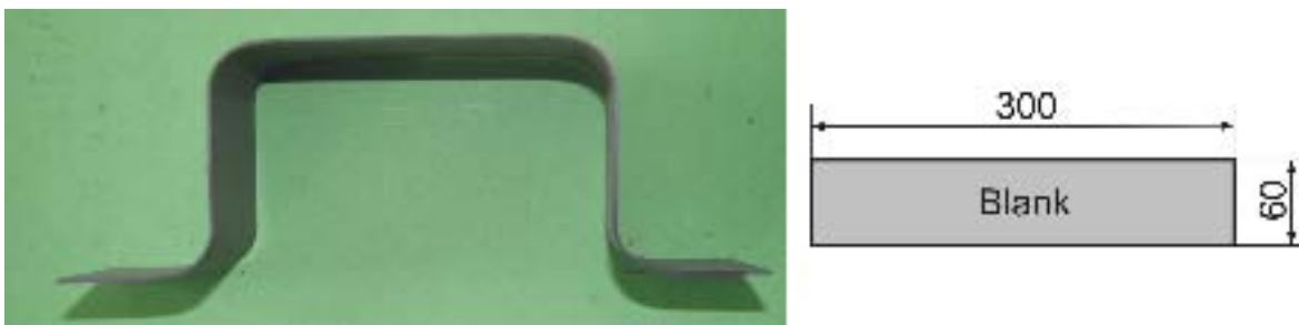
Figure 2. Hot-stamped cap profile and blank dimensions.
