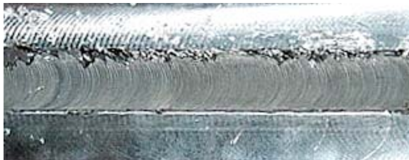
Figure 4: Top view of the FSW on the mill annealed Ti-6Al-4V plate.
