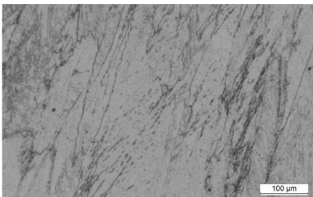
Figure 7. Austenite microstructure after quenching (1420°C-1150°C condition).
