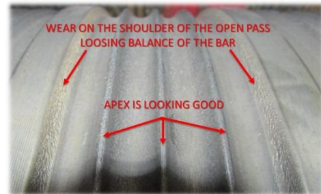
Figure 7: dog bone pass of stand 15 after rolling 2200 tons 4x10mm rebar
