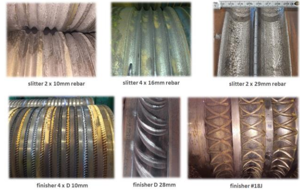
Figure 2: rolling application ULTIMA ® successfully has been tested
