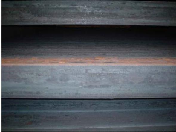
**Figure 5.** Detail of surface of billets cast with LCB 426 (B)
