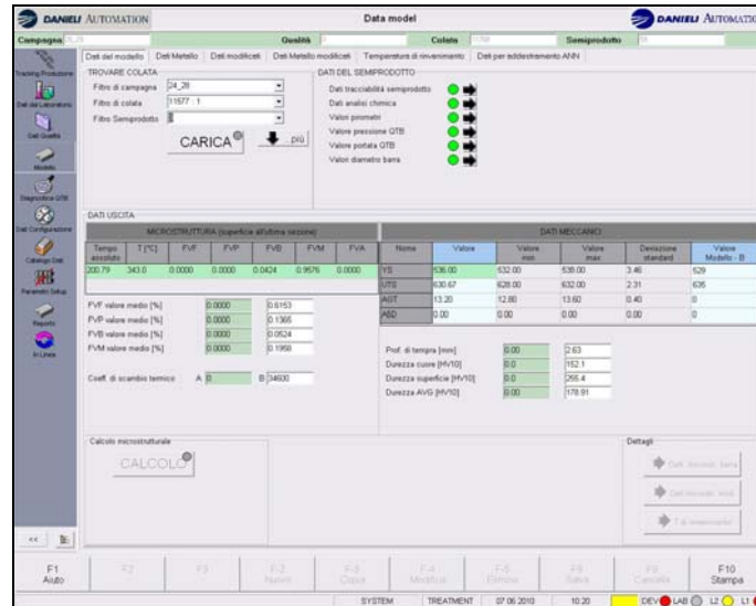
Figure 8: Prediction of microstructure and properties of rebar.
