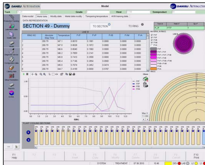
Figure 7: Distribution of different phases along radius of the bar.
