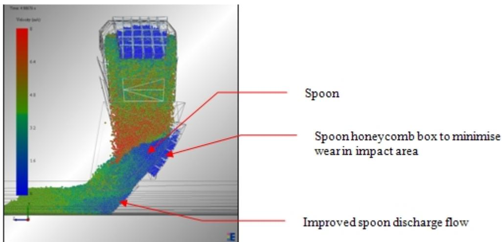
Figure 4. DEM simulation of the new Hood and Spoon Chute (Side View).
