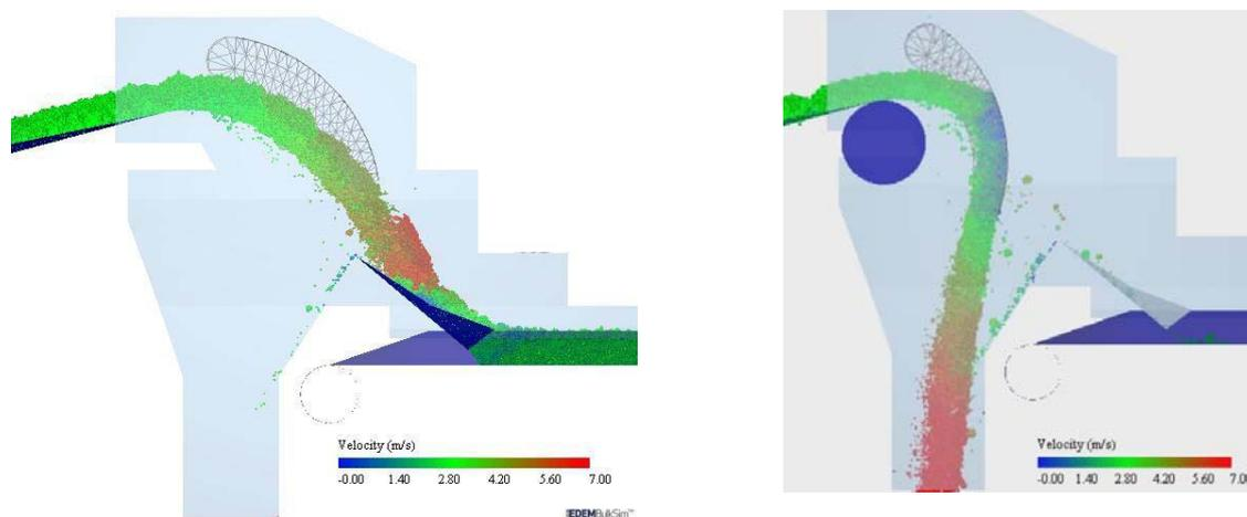
Figure 8. (a) Deflector up for through loading onto collection conveyor, (b) Deflector down for discharge into bin below.
