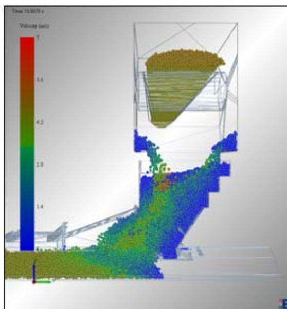
**Figure 2.** DEM simulation of Rock Box Chute, highlighting choking and low velocity loading.
