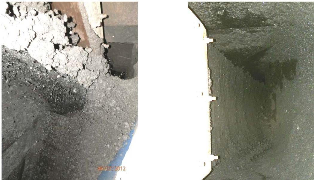
**Figure 10.** (a) Detail of trajectory, through loading, (b) Detail of trajectory in contact with deflector, and discharge into bin.
