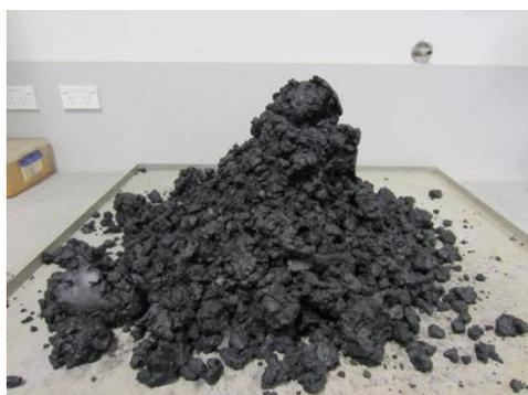
Figure 7. Filtercake appearance (24% wb moisture content).
