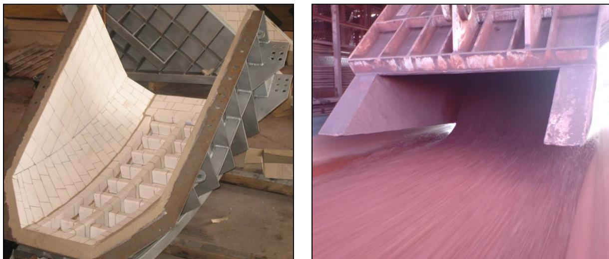
**Figure 5.** (a) Spoon liner installation, (b) Spoon discharge in operating position.
