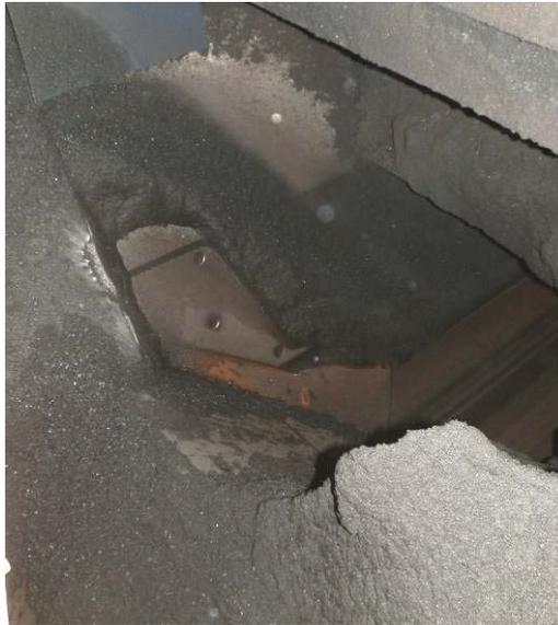
**Figure 11.** Detail of through loading spoon and fine coal buildup directly adjacent the primary trajectory stream.
