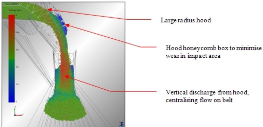
Figure 3. DEM simulation of new Hood and Spoon Chute (front view).
