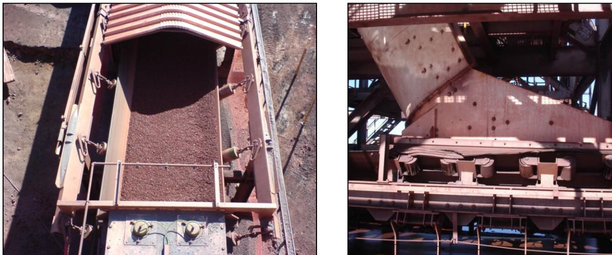
**Figure 1.** (a) Off centre loading of receive conveyor (b) Damaged skirting.
