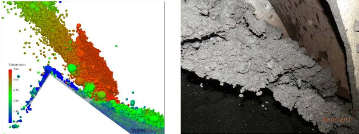
**Figure 9.** (a) Detail of filtercake clumping within trajectory, (b) Coal production trajectory detail adjacent deflector chute.
