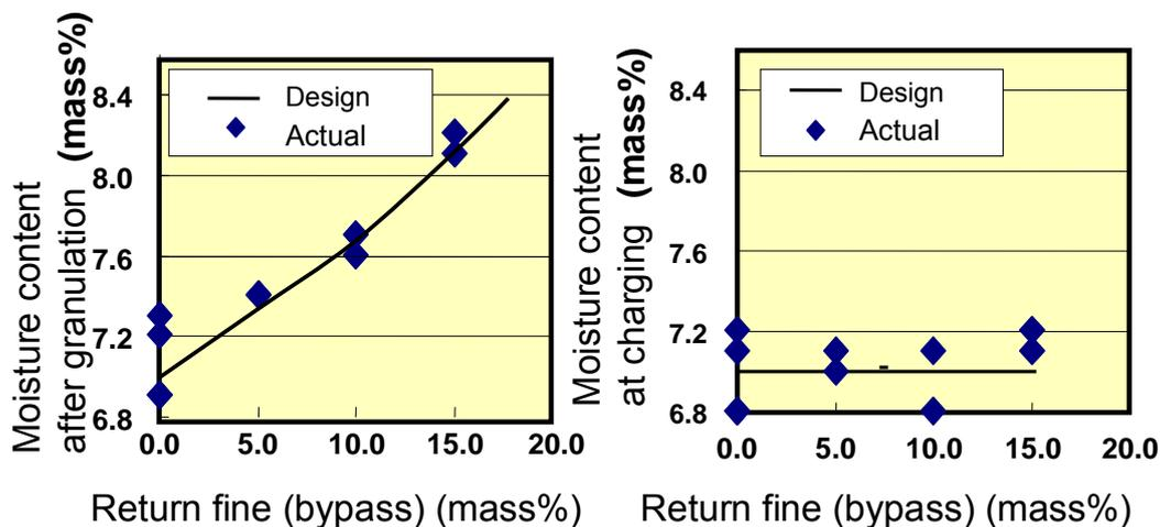
Figure 3. Moisture content in sinter raw materials after granulation and at charging.
