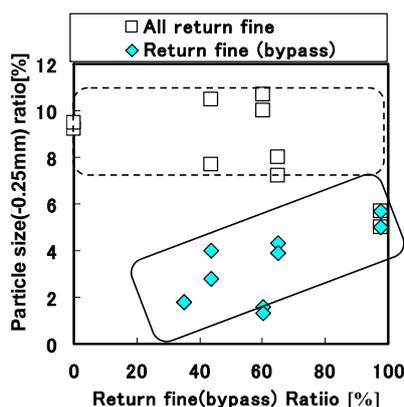
Figure 12. Influence of return fine (bypass) ratio on particle size.
