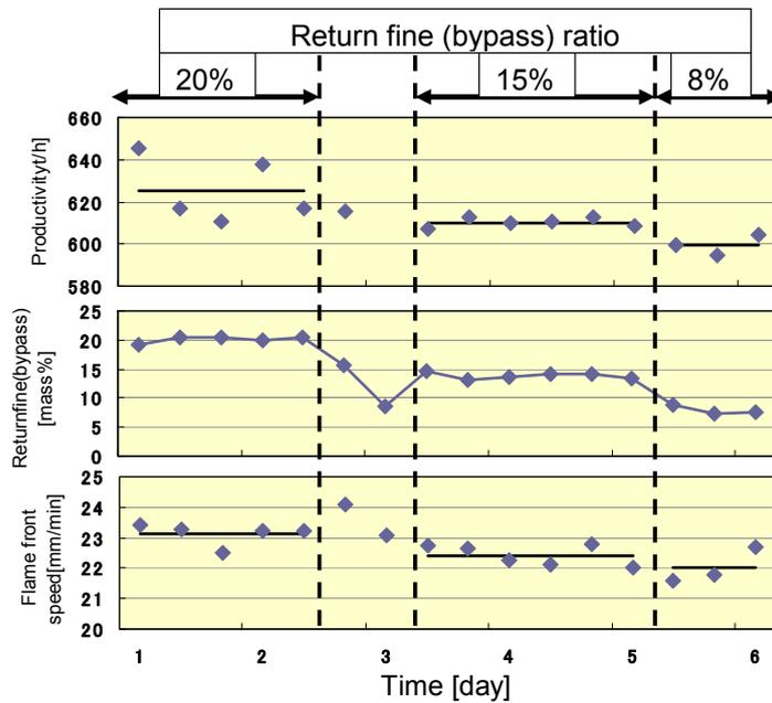
Figure 13. Operational performances at varying return fine bypassing granulation ratio.
