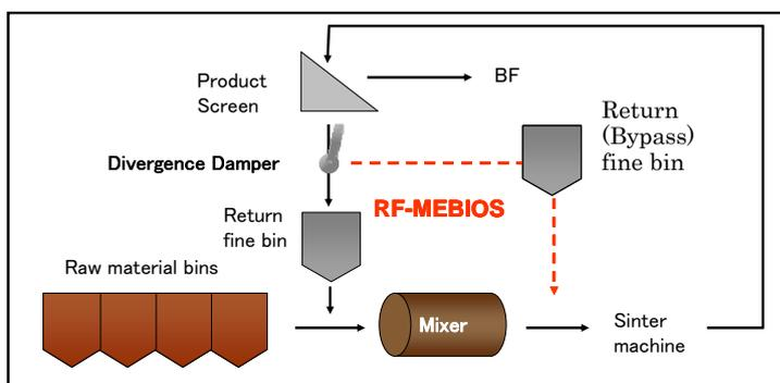
Figure 11. Layout of return fine at commercial sinter plant.
