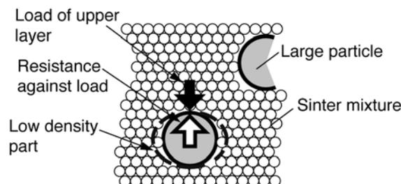
Figure 1. Denser parts and looser ones in the same packed bed of Mebios.<sup>[5]</sup>
