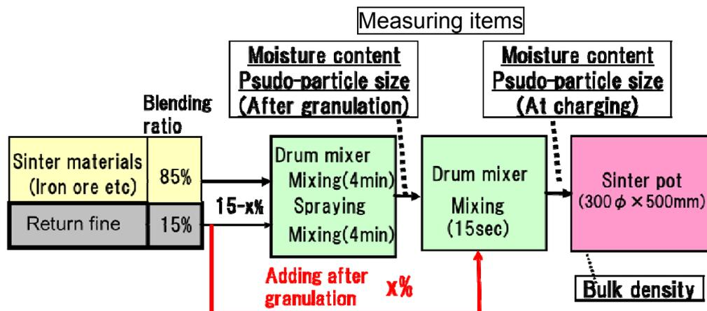
Figure 2. Experimental flow of pot test (300φ).
