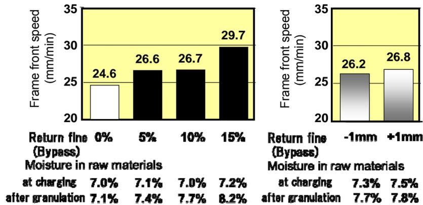
**Figure 6.** Effect of return fine bypass on FFS by return fine bypass.
