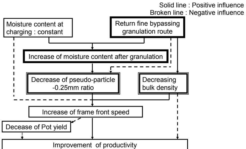
Figure 10. Effect of RF-Mebios (Return fine bypassing granulation route) on improvement of productivity.
