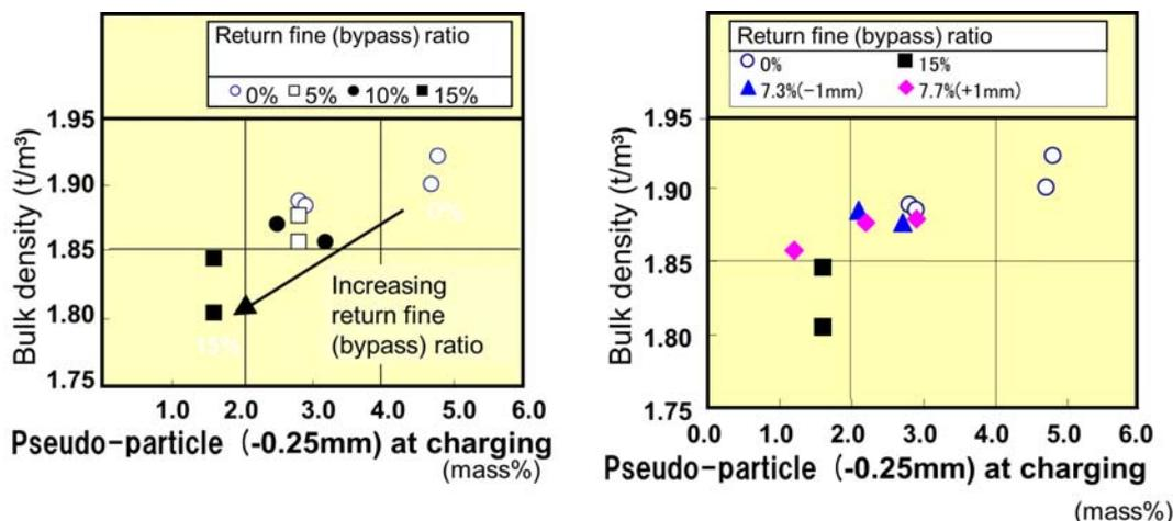
Figure 8. Effect of yield by return fine bypass on bulk density and pseudo-particle size.
