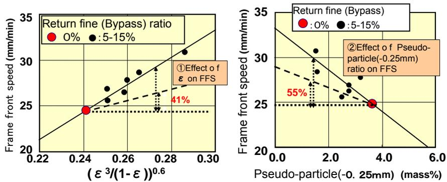
Figure 9. Quantitative analysis for FFS increase by pore ratio and pseudo-particle size.
