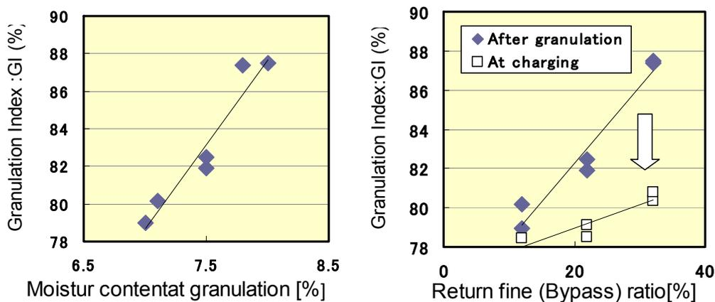
Figure 14. Increasing GI by high moisture content at return fine bypassing granulation.
